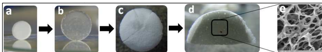
Figure 3.7: Process of pore formation: (a) PEG-PU-1.0HT Xerogel, (b) PEG-PU-1.0HT Hydrogel, (c) Liquid Nitrogen Quenched PEG-PU-1.0HT Hydrogel (d) Freeze
