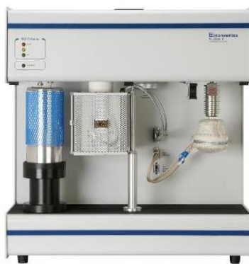
Fig. 2.7 Micromeritics Autochem 2920 used for TPD and TPR study.
