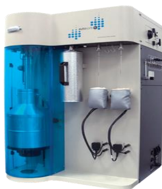
Fig. 2.2 Quantachrome Autosorb IQ instrument used for N_2 physisorption and H_2 chemisorption.
