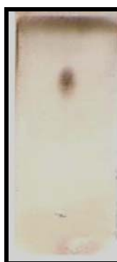
Fig. 3.7: Thin layer chromatography of esterified product (LNNSLME) using silica gel GF254 plates showing single spot
