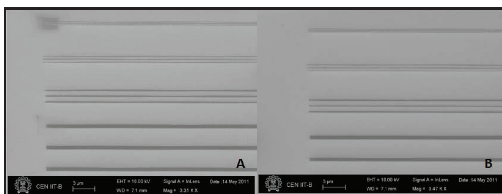
Figure 5.9: SEM images of A) G_1 -Tris-epoxide and B) G_1 -Bis-epoxide EBL pattern Line thickness 500, 200, 100 and 50 nm bottom upward.
