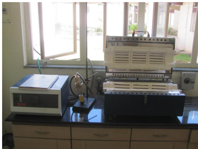
Fig. 2.1 Photo of split-tube furnace
