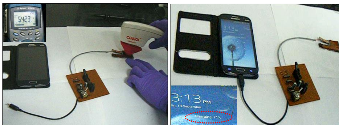
Figure 5.10: Images showing the ability of the device to charge a mobile: The image on the left shows the powering of the device with a vibrator (the voltage is also reflected); and the image on the right shows that mobile charging could be initiated.
