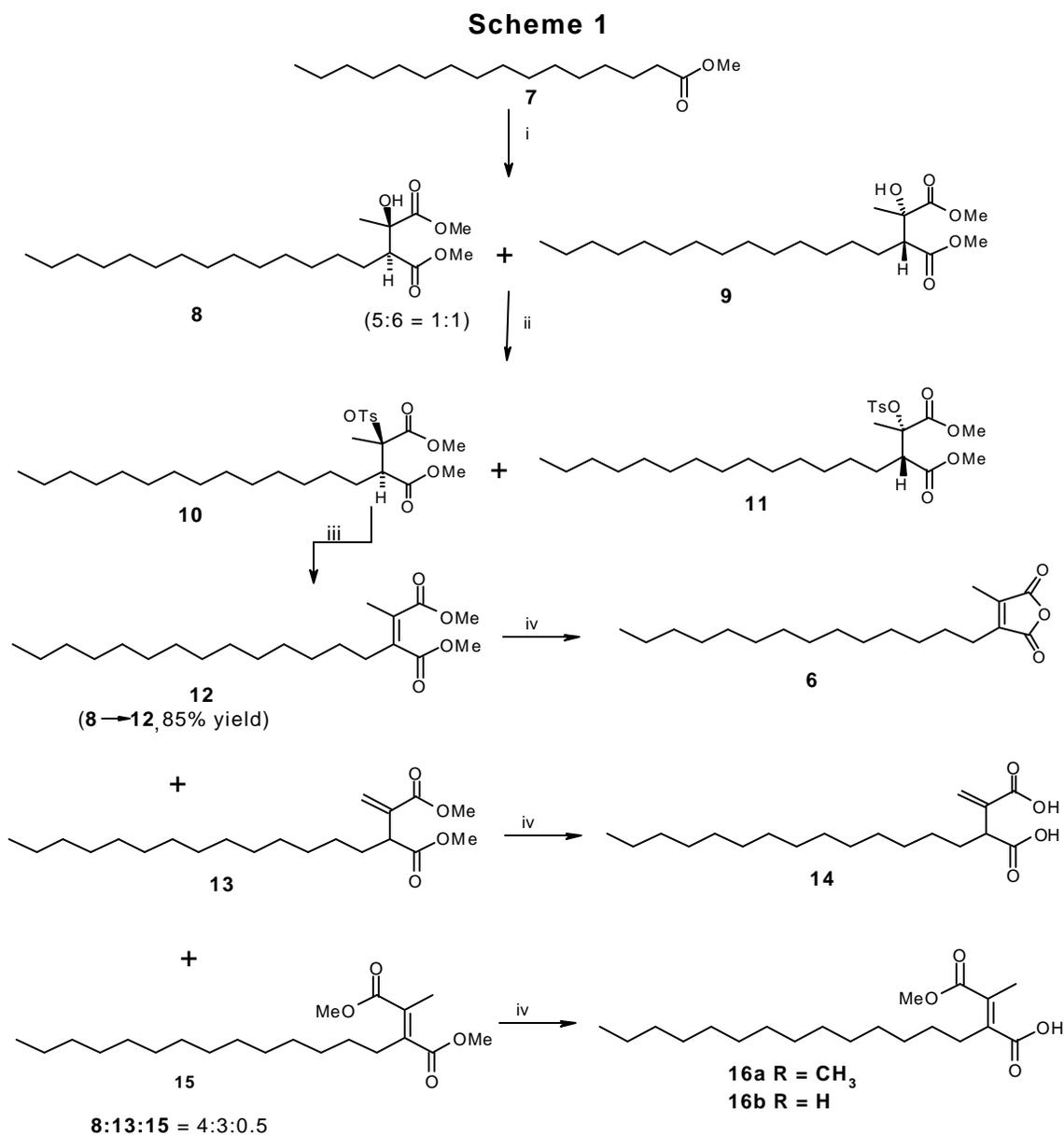
**Scheme 1:** (i) LDA, THF, -78 to -10 °C, methyl pyruvate; (ii) CH<sub>2</sub>Cl<sub>2</sub>, pyridine, 40 °C, 2,6-Di-*tert*-butyl-4-methylpyridine, *p*-toluenesulfonic anhydride; (iii) Toluene, DBU, reflux (iv) a. 1N NaOH-CH<sub>3</sub>OH-THF-H<sub>2</sub>O, 80 °C; b. 4N HCl
