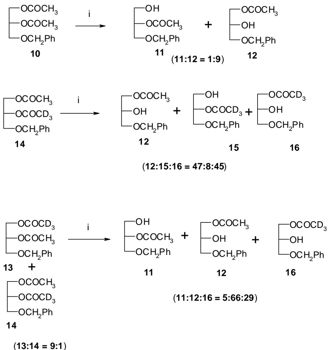
i) PLAP,  $\text{C}_6\text{H}_6$ :Petroleum ether (2:1), 50 mM sodium phosphate buffer pH 8.0 37°C
