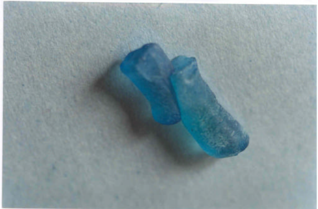
Figure 7.3: Initial stages of healing, formation of thick weld line
