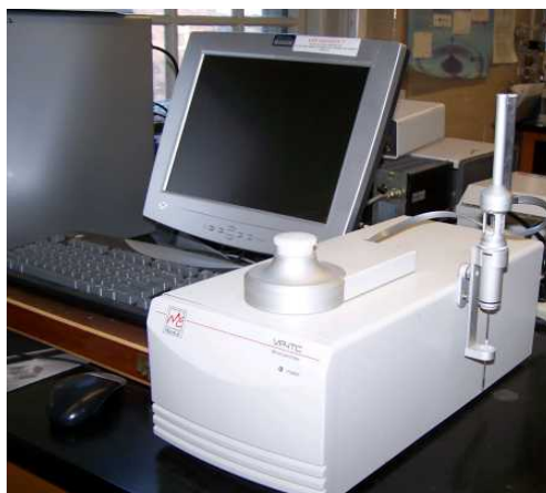
Fig. 3.1: A typical isothermal titration calorimeter (VP-ITC, LLC Microcal 2000)
