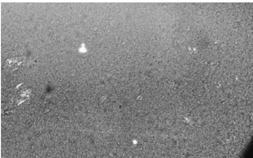
Figure 4.3.6: Optical Micrograph of PN5 crystallized at 152 °C. Magnification 32X
