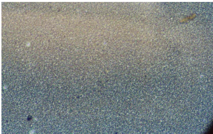
Figure 3.2.6: Optical Micrograph of PNC5 crystallized at 152 °C. Magnification 32X
