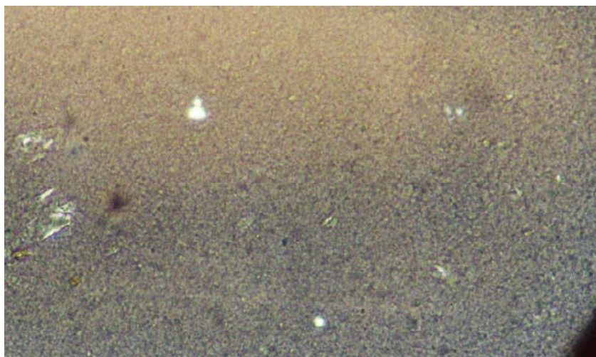
Figure 4.2.6: Optical Micrograph of PN5 crystallized at 152 °C. Magnification 32X
