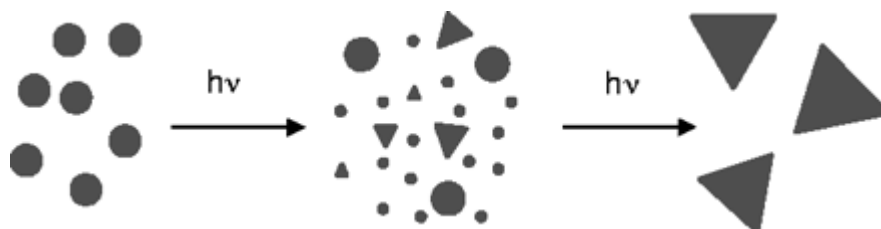
Figure 1.5: Schematic of photoinduced conversion of silver nanospheres to nanoprisms. [Adopted from 25d].
