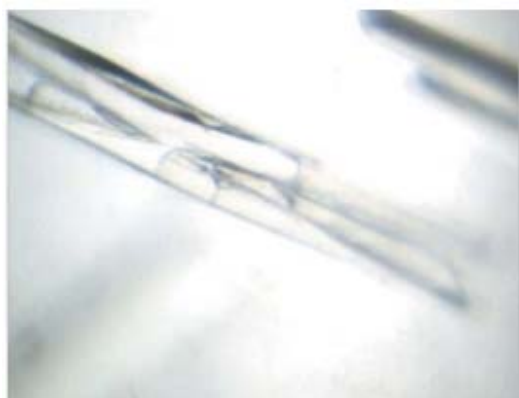
Fig. 4 Crystals of native TSC grown in crystallization condition no. 18 (0.2 M magnesium acetate, 0.1 M sodium cacodylate pH 6.5, 20% PEG 8000) of Crystal screen 1 from Hampton Research.
