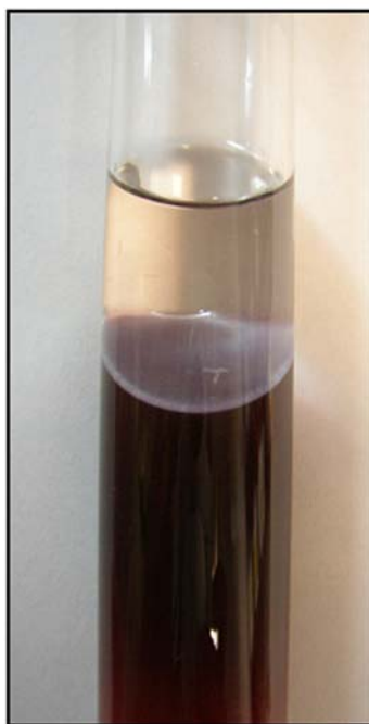
Figure 3.10: Test-tube showing the thin film of gold sheet formed at the interface of ODA in toluene and a mixture of \text{HAuCl}_4 and Keggin ion (PTA) after UV irradiation.
