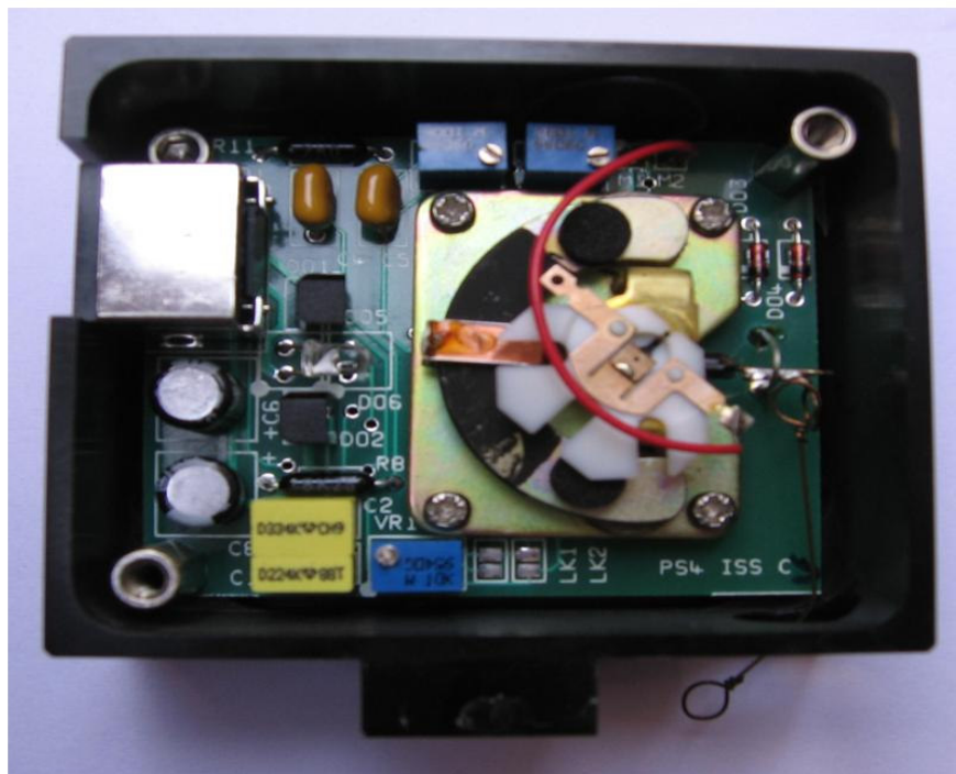
Figure 3.4-III Pressure sensor with signal conditioning circuitry
