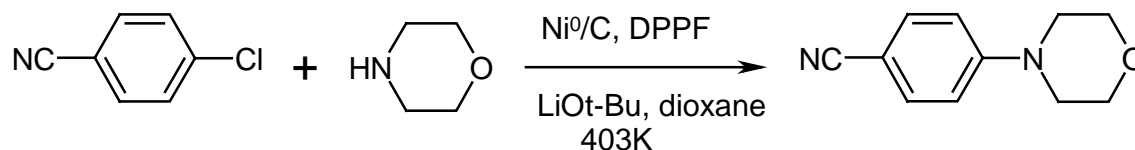
Scheme 1.13: Ni-catalyzed amination of chlorobenzene with morpholine
