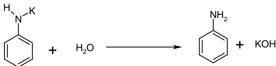
Scheme 3.11: Reaction with potassium salt of aniline with water
