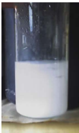
Figure 5.2 : Pictorial view of emulsion of styrene and divinyl benzene formed
