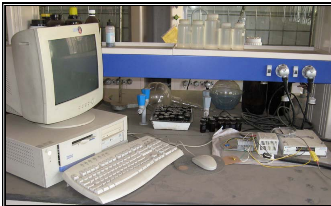
Figure 4.4 Online data acquisition system used for H 2 S abatement
