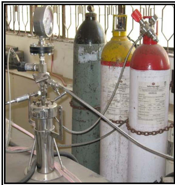
Figure 4.2 H 2 S gas cylinders along with gas reservoir
