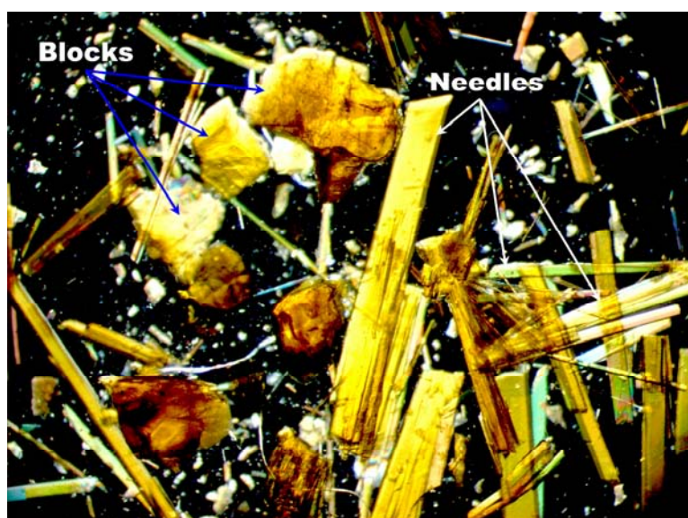
Figure 2.26: Photomicrographs of polymorphs of Fc(CA) complex, blocks ( Form I ) and needles ( Form II ).
