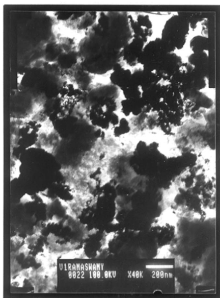
FIGURE 2.4 TEM OF FRESH 5 % Rh/C CATALYST
