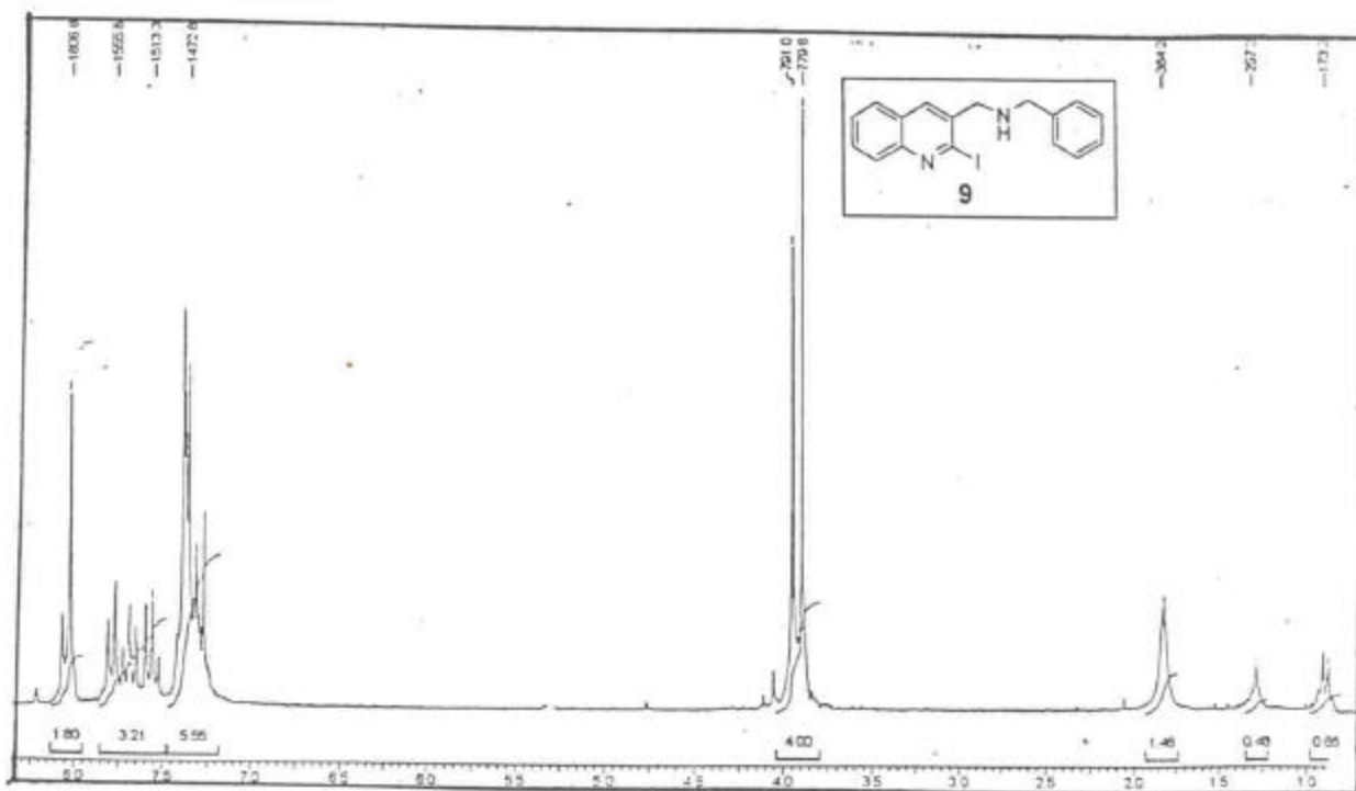
^1\text{H-NMR} spectrum of compound [9]. ( \text{CDCl}_3 , 200 MHz)
