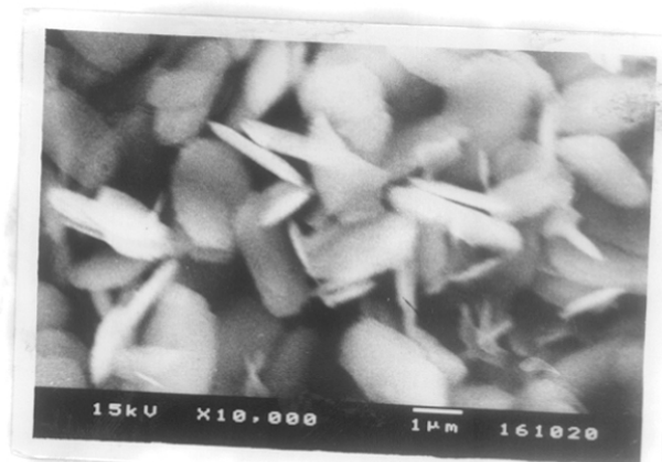
Fig.2.13 Scanning electron micrographs of samples with Si/Al molar ratio of 83 (micrograph 'a'), 257 (b) and >3000 (c).
