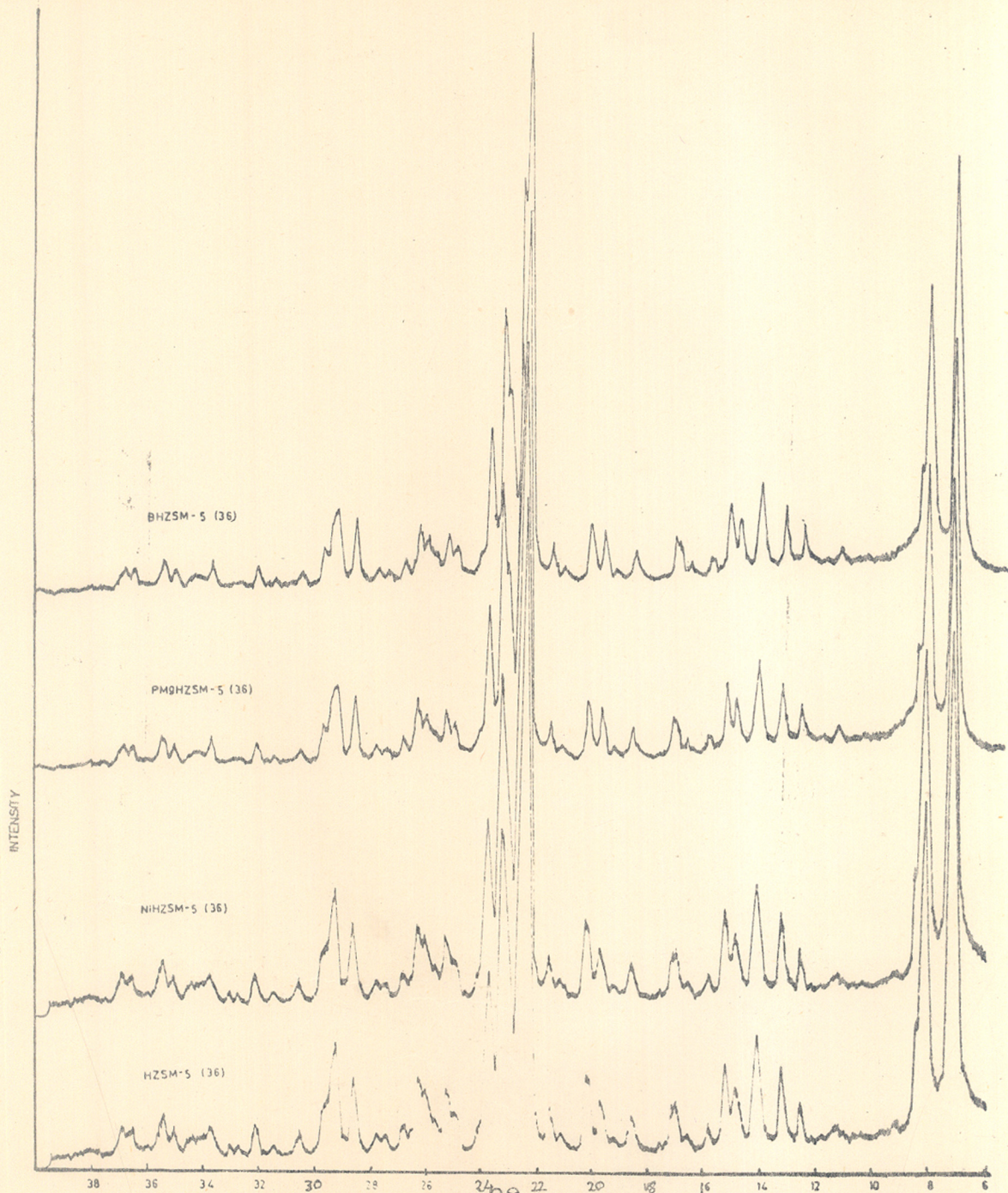
FIG.2.1 X-RAY DIFFRACTOGRAMS OF HZSM-5 AND MODIFIED HZSM-5 ZEOLITES. THE NOS. IN BRACKETS REFER TO \text{SiO}_2/\text{Al}_2\text{O}_3 RATIO.
