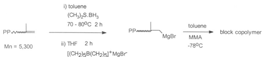
Scheme 1.18 Synthesis of polyethylene-block-polymethyl methacrylate copolymer
