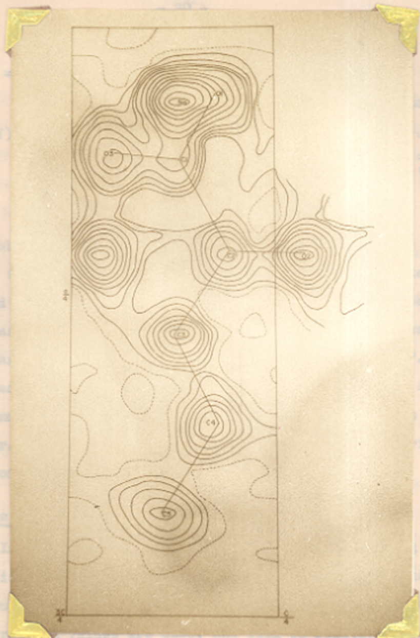
FIG. 7: ELECTRON DENSITY PROJECTION ON (010). CONTOURS ARE DRAWN AT INTERVALS OF 1 e/\text{\AA}^2 . FIRST FIVE CONTOURS AROUND \text{Na}^+ , \text{O}_1 AND \text{O}_3 ATOMS ARE AT 1 e/\text{\AA}^2 INTERVALS AND THEN ALTERNATE CONTOURS ARE DRAWN. 1 e/\text{\AA}^2 CONTOUR IS DASHED.
