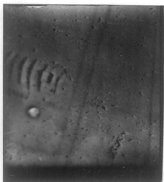
Fig. 37. A scratch re-polished with rouge after etching.
