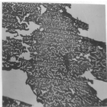
Fig. 59. Electron micrograph of a silver film deposited on a rocksalt cleavage face at room temperature, and heated on the substrate to 570^{\circ}\text{C} . 5000 x.
