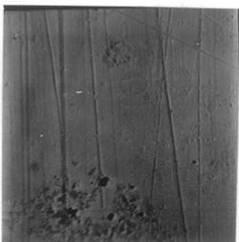
Fig. 33. Shaded formvar replica of scratches on a glass slide, made by rubbing with elutriated diamond dust, by electron microscopy. 10,000 x.
