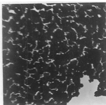
Fig. 60. Electron micrograph of a silver film deposited on a rocksalt cleavage face at 250^{\circ}\text{C} ., 5000 x.
