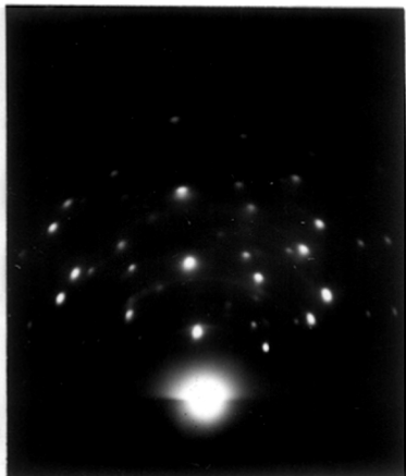
Fig. 12. (100)-face; 2 min. at 200°C. Crystalline film; various orientation.
