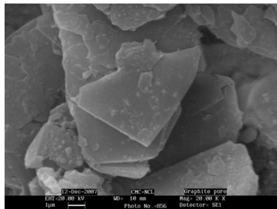
**Figure 3.1.9.** SEM picture of pure graphite
