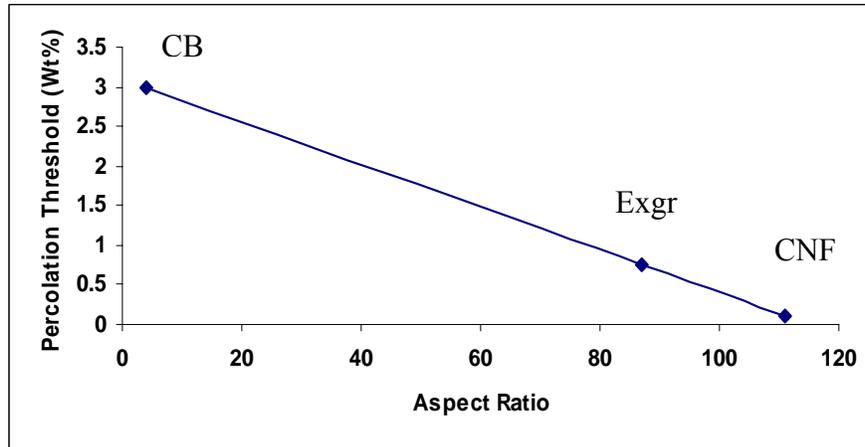
**Figure 5.5.** Aspect ratio of second filler vs percolation threshold
