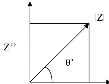
**Figure. 1.11.** Impedance resolved in to real and imaginary parts
