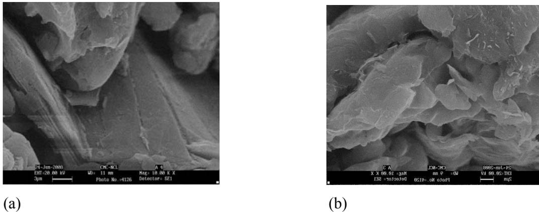
**Figure 3.3.8.** SEM pictures of PES-7 wt% ExGr a) unsintered b) sintered sample
