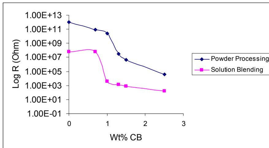
**Figure 3.1.4.** Effect of preparation routes on the through plane resistance of PES-graphite-CB composites (Thickness 5 mm and area 1 cm<sup>2</sup>)
