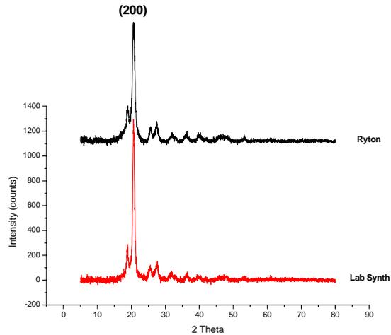
**Figure 4.5.7.** XRD pattern comparison between synthesized and commercial PPS
