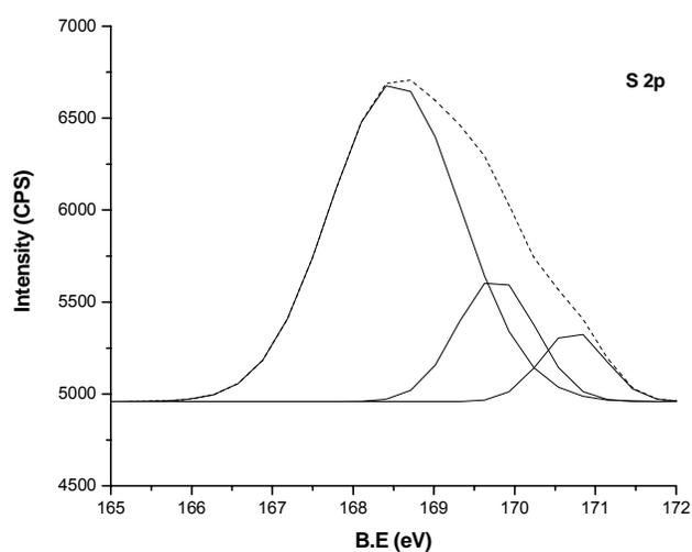
**Figure 3.1.18.** S 2p core level spectrum of PES mixed with graphite
