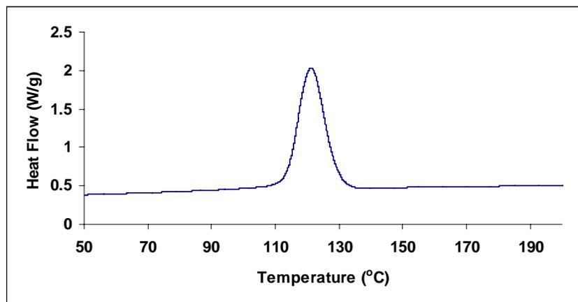
**Figure 5.4.10.** DSC cooling curve of PP-7 wt% graphite-1 wt% CNF
