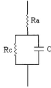
**Figure. 1.12.** Equivalent circuit of CPCs
