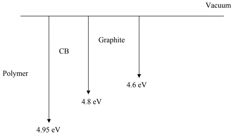
**Figure 3.1.27.** Work function diagram of fillers
