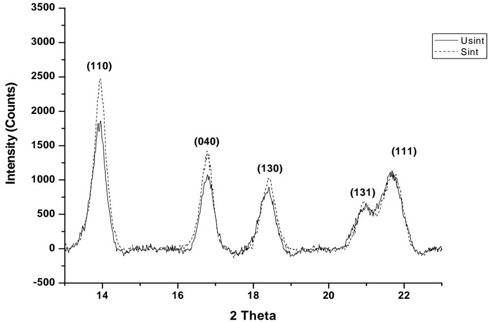
**Figure 5.2.5.** XRD pattern of PP part of PP-40 wt% graphite
