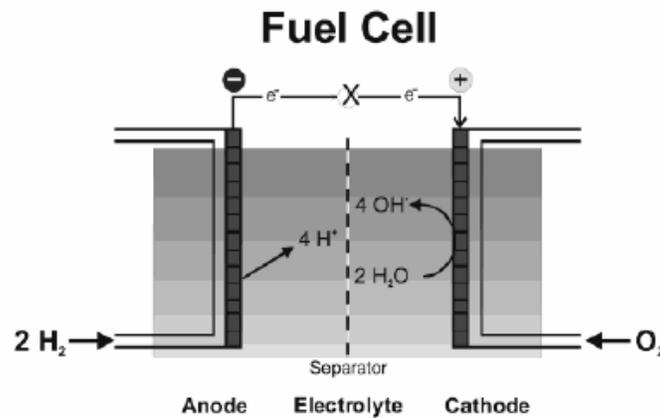
**Figure. 1.15.** Typical Fuel cell operation
