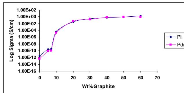
Figure 4.2.1. DC conductivity of PPS-graphite composites
