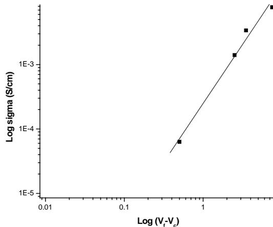
**Figure 4.3.2.** Plot for obtaining percolation exponent in PPS-ExGr composites
