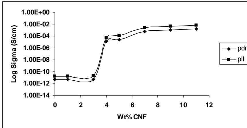
**Figure 3.2.2.** DC conductivity of PES-CNF composites
