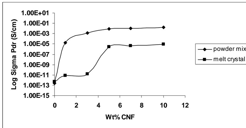
**Figure 5.8.2.** Effect of processing route on the through plane conductivity of PP-CNF binary composites
