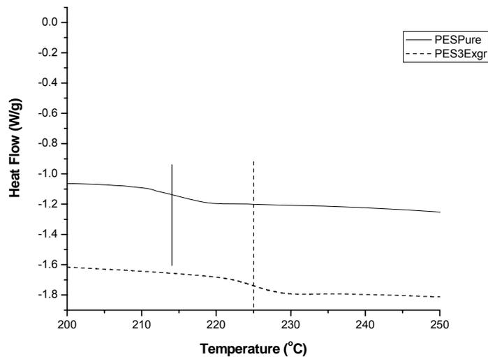
**Figure 3.3.10.** DSC curves of PES and PES-3 wt% ExGr composite
