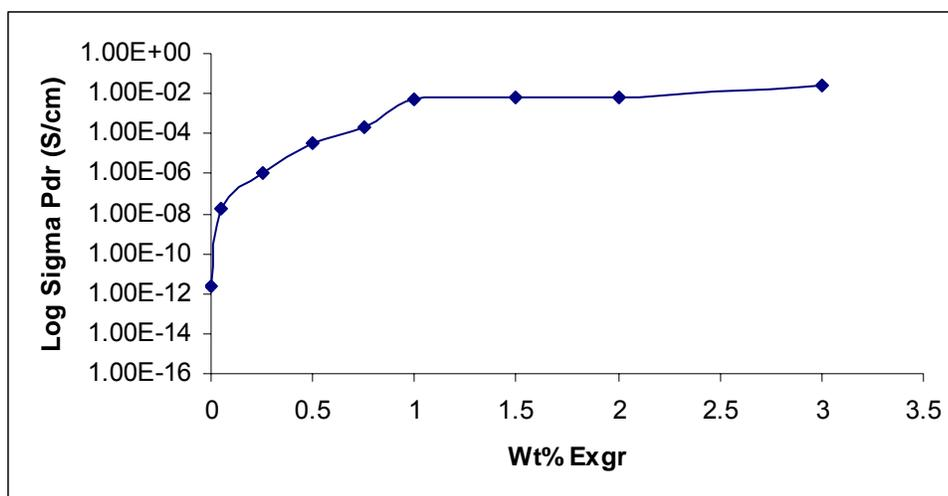
**Figure 3.3.11.** DC conductivity of PES-7 wt% graphite-x wt% ExGr composites
