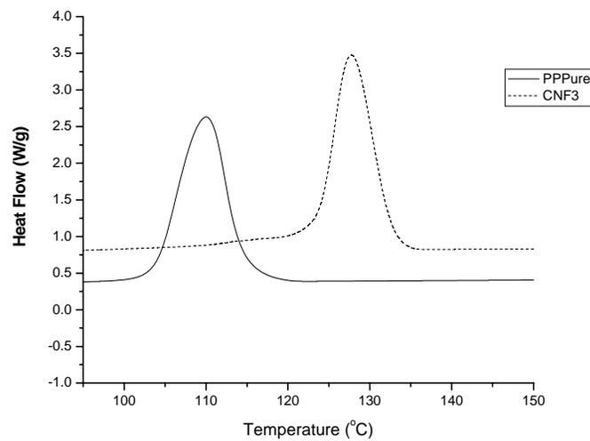
**Figure 5.4.9.** DSC cooling curve of pure PP and PP-3 wt% CNF composite
