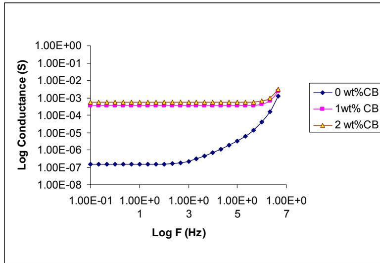
**Figure 3.1.20.** AC conductance of PES-7 wt% graphite-x wt% CB (x=0,1,2)
