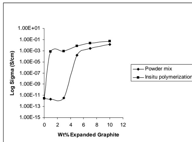
**Figure 4.5.10.** Through plane conductivity of synthesized PPS-ExGr composites
