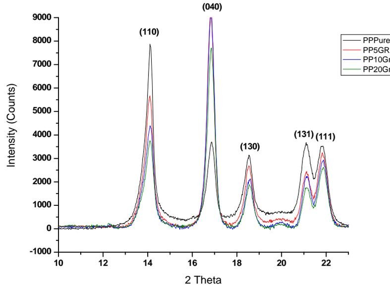
**Figure 5.6.1.** XRD patterns of melt crystallized PP-graphite composites
