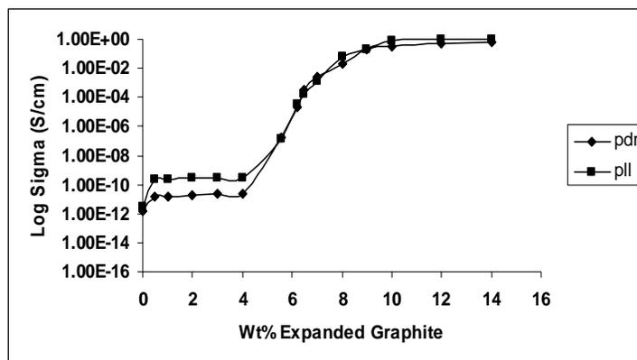
**Figure 5.3.1.** DC conductivity of powder mixed PP-ExGr composites
