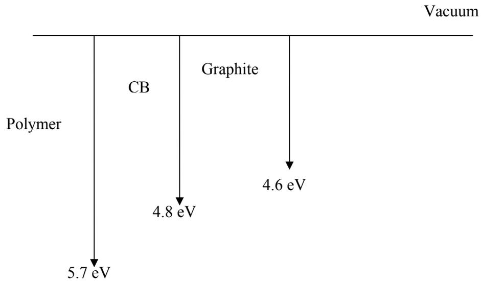
**Figure 5.2.10.** Work function diagram of components in hybrid composites
