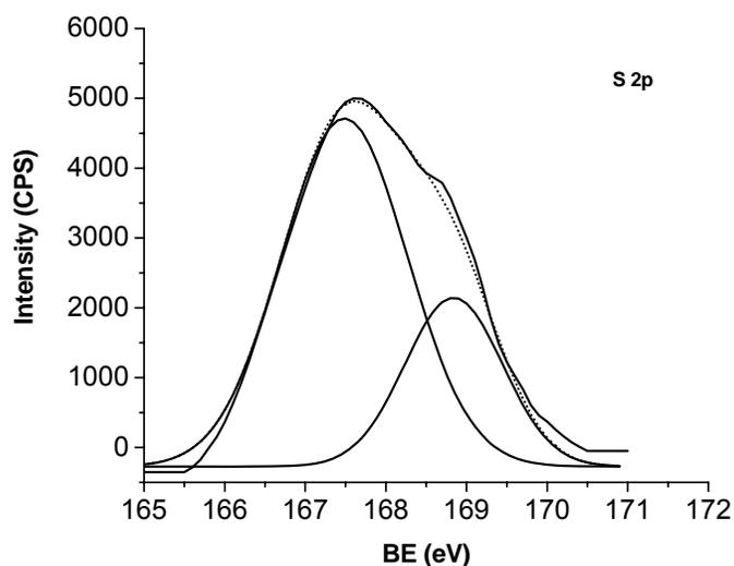
**Figure 3.1.17.** S 2p Core level spectrum of PES
