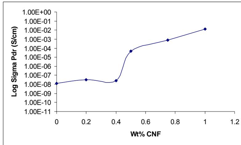
**Figure 3.2.9.** Through plane conductivity of PES-7 wt% graphite-x wt% CNF
