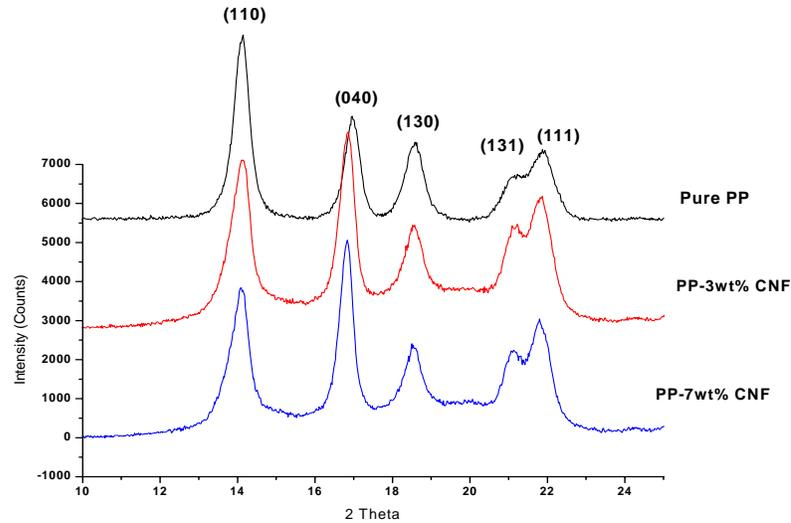
**Figure 5.8.3.** XRD patterns of melt crystallized PP, PP-3 wt% CNF and PP-7wt% CNF
