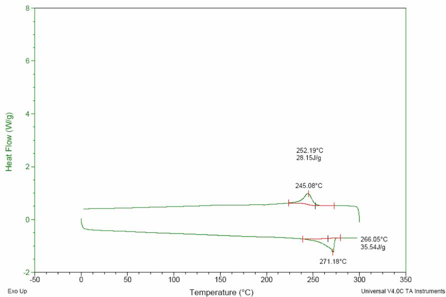
**Figure 4.5.8.** DSC of synthesized PPS
