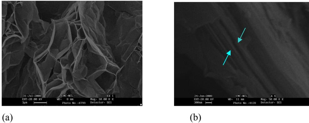
**Figure 3.3.7.** SEM pictures of a) pure ExGr b) PES-10 wt% ExGr
