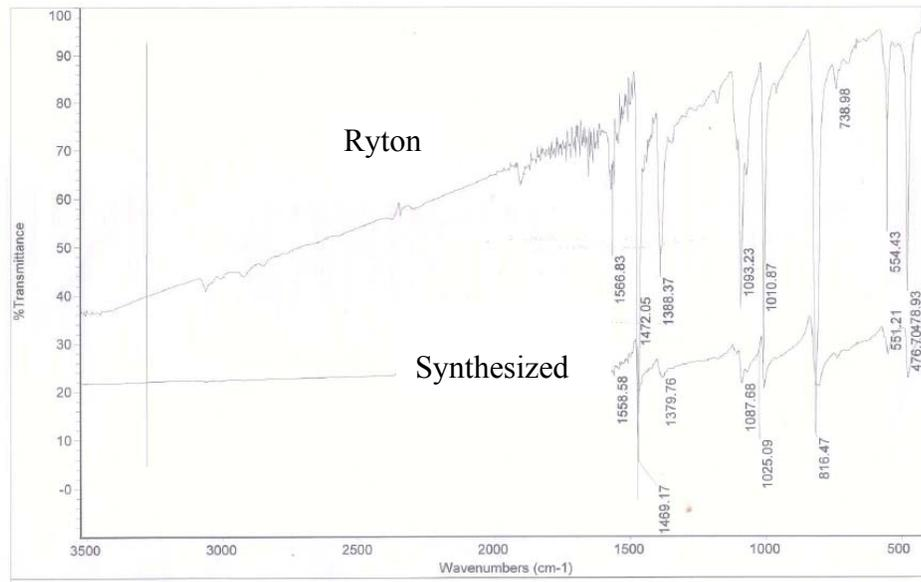
**Figure 4.5.9.** IR of Ryton and synthesized PPS
