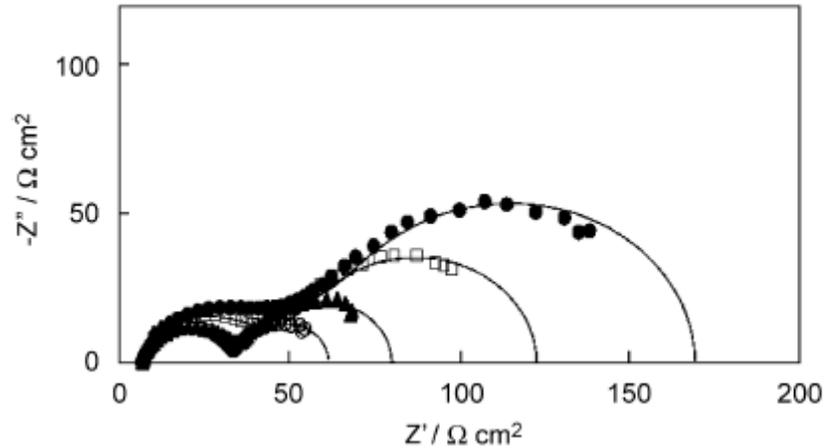
**Figure 1.13.** Impedance plot of oxygen reduction reaction at Pt/Nafion interface
