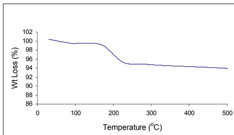
**Figure 3.1.14.** TGA of DPS-38 wt% graphite
