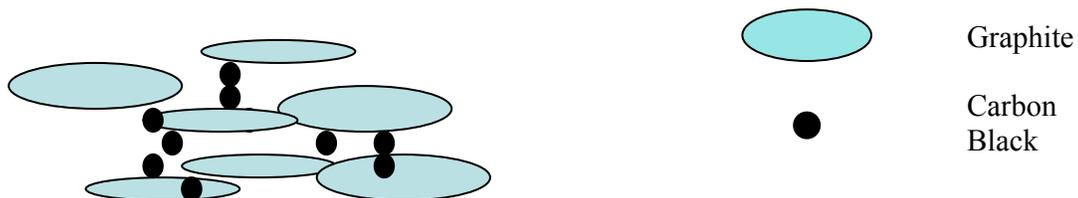
**Figure 3.1.23.** Model of hybrid composites
