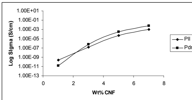
**Figure 3.2.5.** Conductivity variation of PES-CNF after sintering
