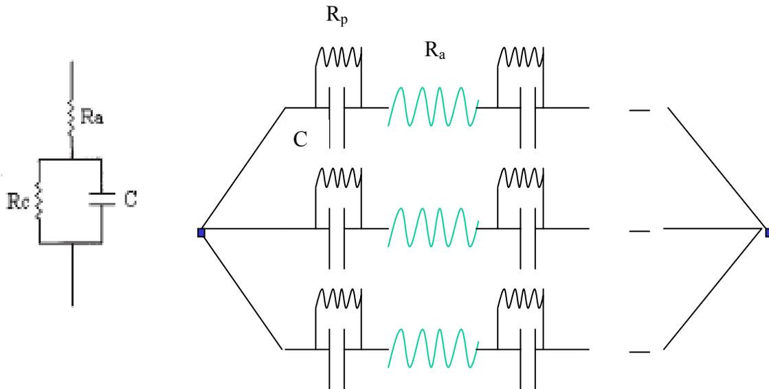
**Figure 4.2.12.** Model of conducting polymer composites
