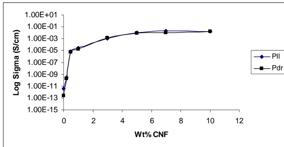
**Figure 5.4.1.** DC conductivity variation of PP-CNF powder mixed composites
