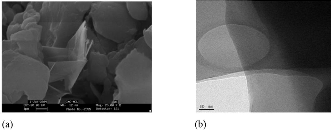
**Figure 4.4.12.** a) SEM b) TEM pictures of expanded graphite
