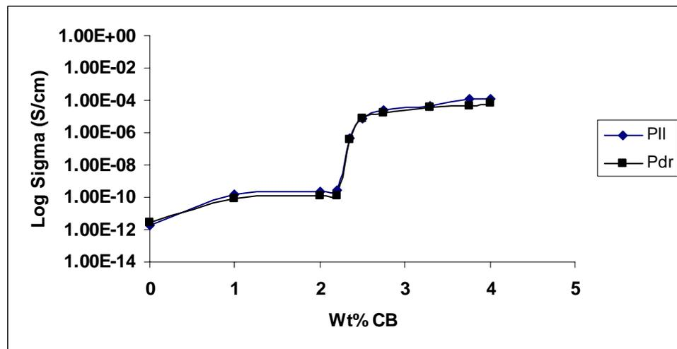
**Figure 5.2.6.** DC conductivity of PP-7 wt% graphite-CB hybrid composites
