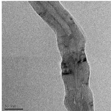
**Figure 4.4.5.** TEM picture of CNF mixed in PPS
