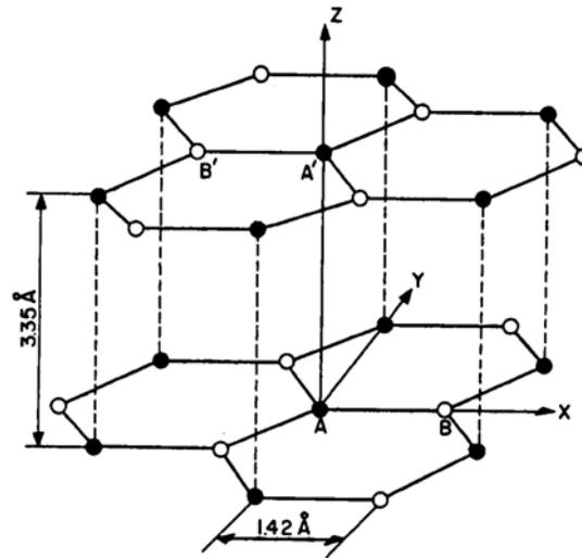
**Figure. 3.1.1.** Crystal structure of graphite
