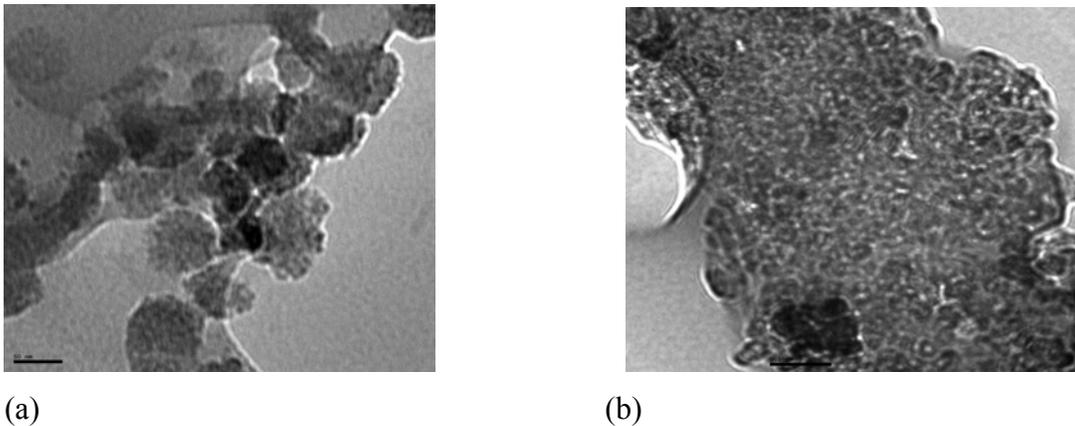
**Figure 3.1.8.** TEM pictures of solution blended PES-7 wt% graphite a) unsintered b) sintered samples
