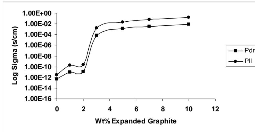
**Figure 4.3.1.** DC conductivity of PPS-ExGr composites
