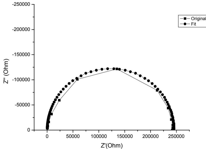
**Figure 3.1.26.** Impedance plot of PES-7 wt% graphite-2.5 wt% CB powder mixed sample
