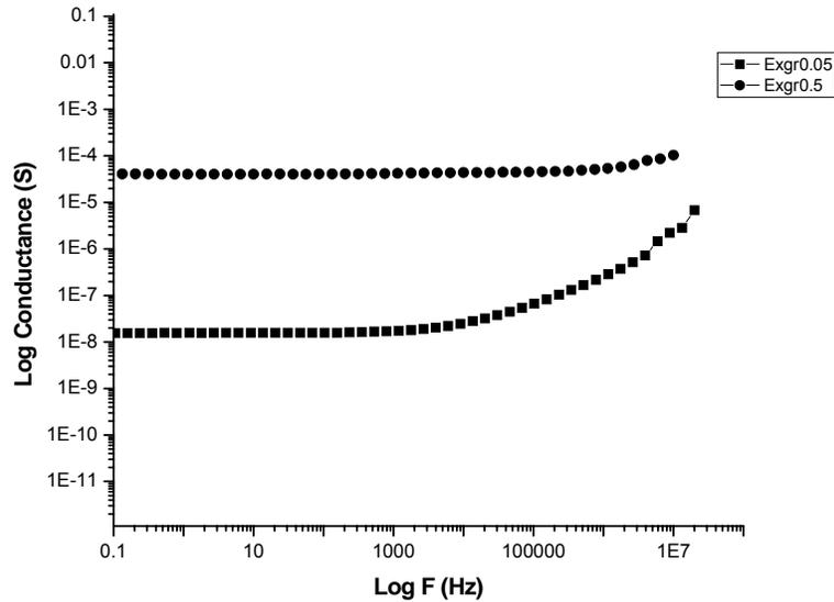
**Figure 3.3.12.** AC conductance of PES-7 wt% graphite-x wt% ExGr (X=0.05, 0.5)
