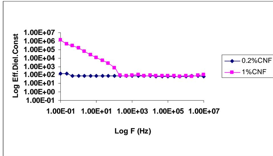
**Figure 5.4.6.** Effective dielectric constant vs. frequency of PP-CNF composites
