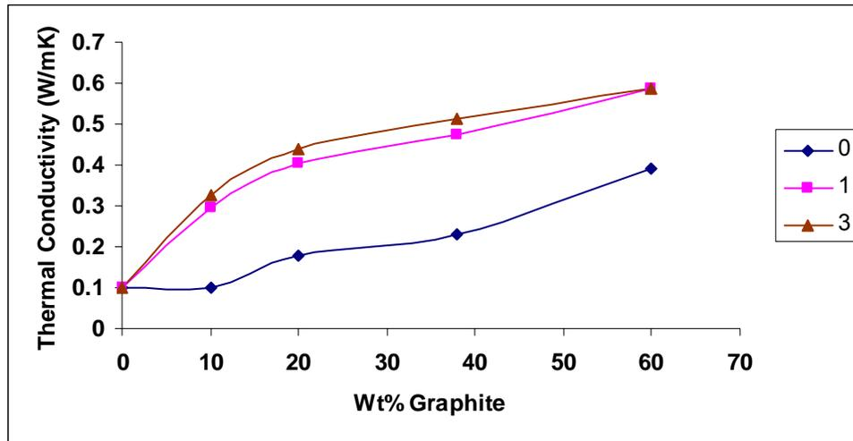
**Figure 3.5.1.** Thermal conductivity of PES-graphite-CB composites
