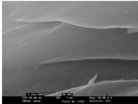
**Figure 4.5.3.** SEM picture of cross section of PPS-3 wt% ExGr melt crystallized sample
