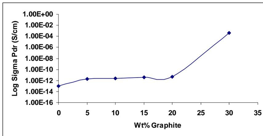
**Figure 5.6.** Through plane conductivity of melt crystallized PP-graphite composites
