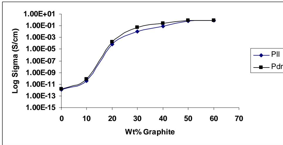
Figure 5.2.2. DC conductivity of PP-graphite composites after sintering
