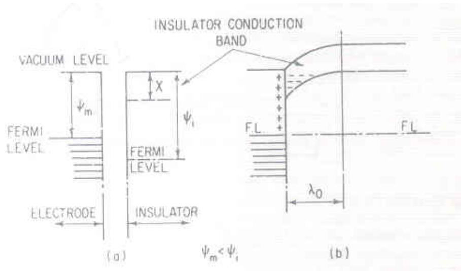
**Figure. 1.7.** Band diagram for Ohmic contact
