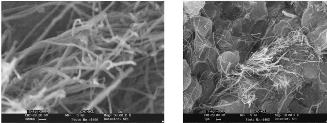
**Figure 5.4.3.** SEM pictures of cross section of PP-7 wt% CNF composite
