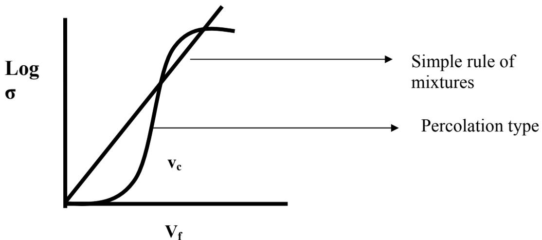
**Figure. 1.4.** Electrical conductivity variation in CPCs
