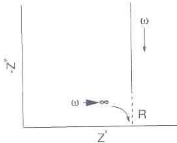
This model can be used to model a metal with undamaged high impedance coatings.
