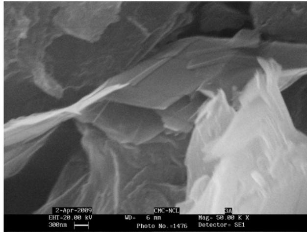
**Figure 5.3.8.** SEM image of cross section of PP-6 wt% ExGr composite
