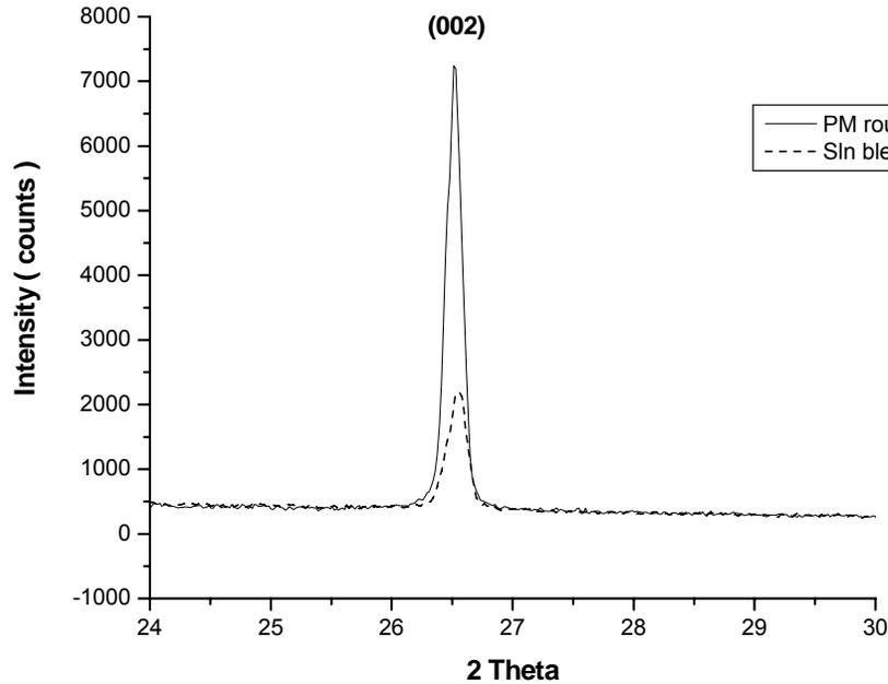
**Figure. 3.1.5.** XRD pattern of PES-7 wt% Graphite prepared by different routes
