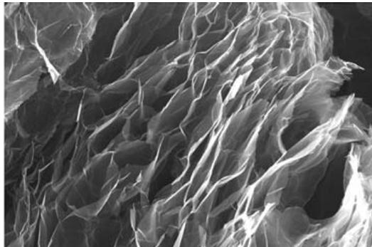
**Figure 3.3.1.** SEM picture of expanded graphite
