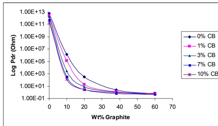
**Figure 3.1.3.** Through plane resistance of solution blended PES-Graphite-CB composites (sample thickness-5 mm, area of cross section-1 cm<sup>2</sup>)
