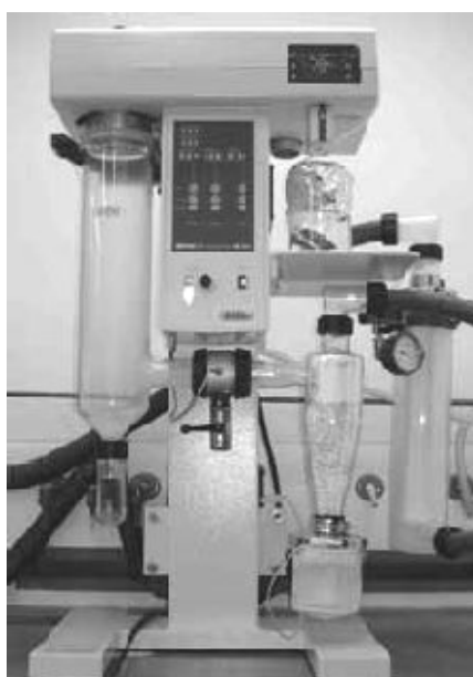
Figure 1.10. Spray drier for the preparation of drug loaded polymer microparticles
