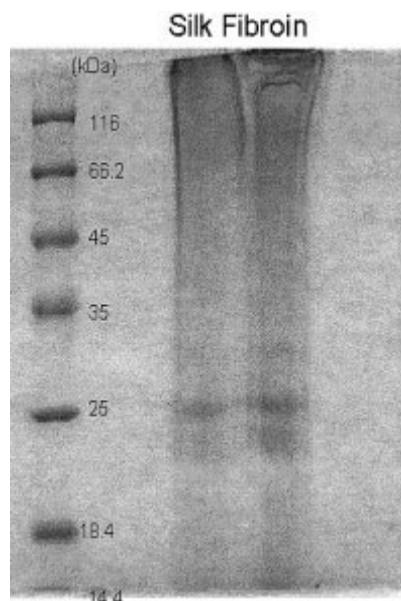
Figure 2.15: SDS gel page of regenerated silk fibroin (Iridag Y. et al [76]; Applied for reproduce permission )
