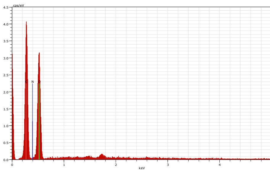
Figure 5.40: EDAX spectrum of 2, 3-diethylimine cellulose-5 showing nitrogen peak
