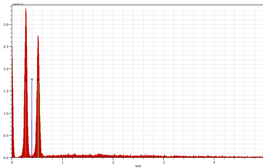
Figure 5.41: EDAX spectrum of 2, 3-dipropyimine cellulose-5 showing nitrogen peak
