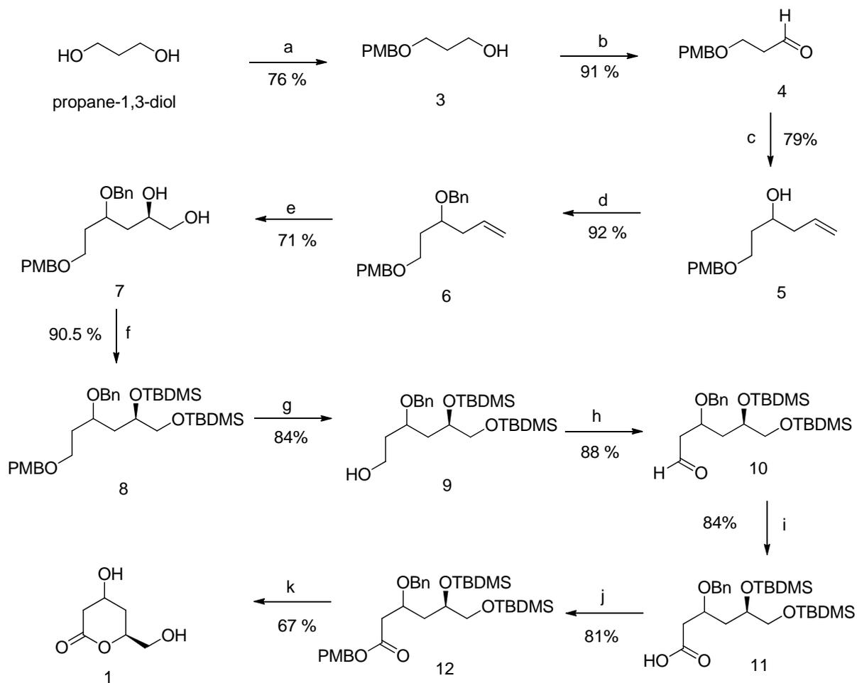
**Scheme 2.** *Reagents and conditions:* (a) NaH, PMB-Cl, DMF; (b) PCC, DCM, RT; (c) Allyl bromide, Zn, THF, aq NH<sub>4</sub>Cl; (d) NaH, BnBr, TBAI, DMF; (e) AD-mix β, <sup>t</sup>BuOH + H<sub>2</sub>O; (f) TBDMS-Cl, imidazole, DCM; (g) DDQ, DCM:H<sub>2</sub>O; (h) PCC, DCM, RT; (i) NaClO<sub>2</sub>, NaH<sub>2</sub>PO<sub>4</sub>, DMSO, H<sub>2</sub>O; (j) PMB-OH, EDCI, DMAP, DCM; (k) TBAF, THF-RT.
