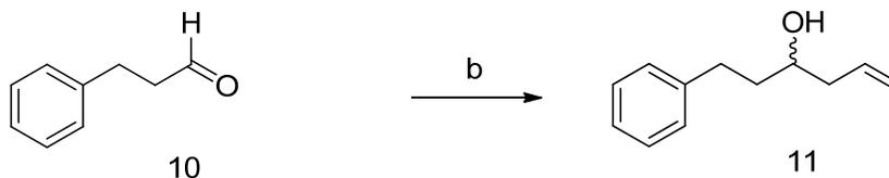
To the stirred solution of **10** (20 gm, 0.149 mole) in THF (200 mL) and aq  $\text{NH}_4\text{Cl}$  (saturated solution 100 mL), zinc (19.08 gm, 0.298 mole, 2 eq) was added slowly in portion. After  $\frac{1}{2}$  hour of stirring, allyl bromide (35.76 gm, 0.298 moles, 2 eq) was added dropwise. The progress of the reaction was monitored by TLC. After completion of the reaction, work up of the reaction was carried out by filtration over celite and
