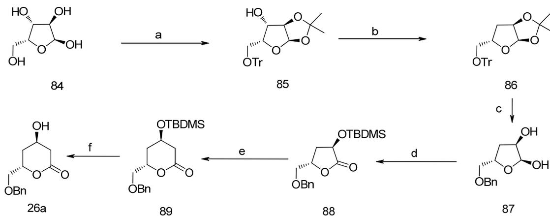
**Scheme 12.** Reagents and conditions: (a) (i) Acetone,  $\text{CuSO}_4$  (anhy), (ii) AcOH, RT, 3. TrCl, Py; (b) (i) NaH,  $\text{CS}_2$ , MeI, THF, (ii)  $\text{Bu}_3\text{SnH}$ , AIBN, Benzene, reflux; (iii)  $\text{H}_2$ , Pd/C, EtOH; (c) (i) NaH, BnBr; (ii) 3.2 M HCl; dioxane (1:1); hr; (d) (i)  $\text{Ag}_2\text{CO}_3$ -celite; (ii) TBDMSCl, imidazole; (e) (i)  $\text{LiCHBr}_2$ , THF,  $-90^\circ\text{C}$ , HCl sat. in  $\text{Et}_2\text{O}$ ; (f) TBAF, THF.
