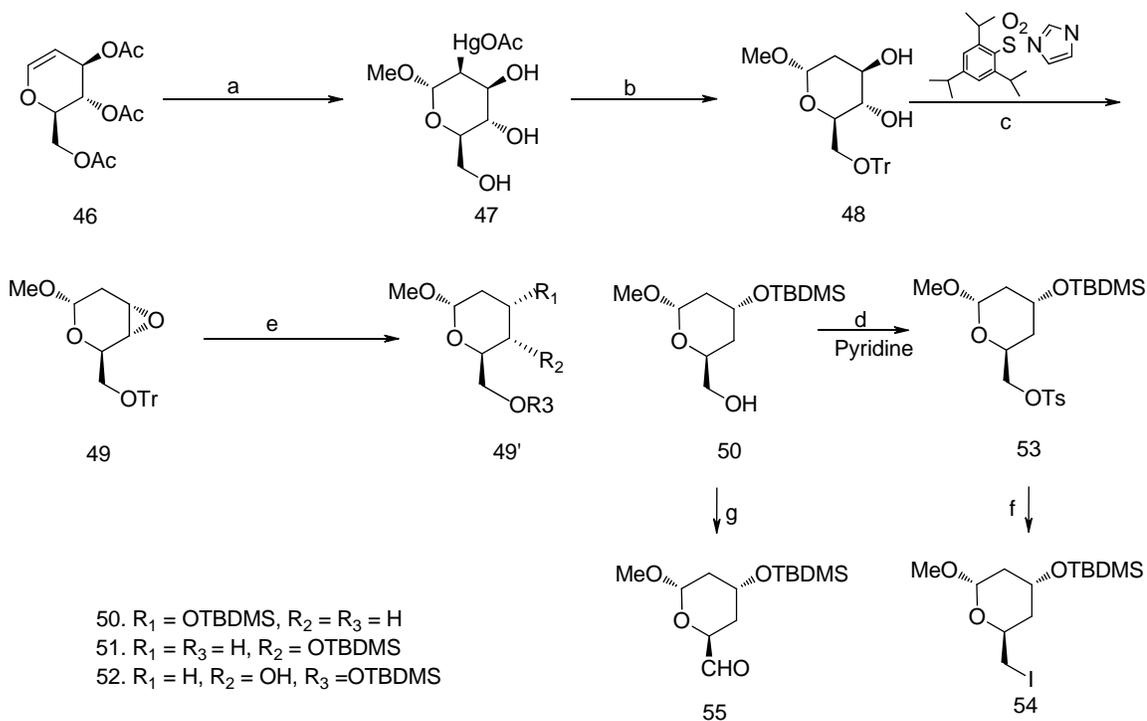
**Scheme 7.** *Reagents and conditions:* (a) (i) NaOMe, MeOH; (ii) Hg(OAc)<sub>2</sub>, THF; (b) (i) NaBH<sub>4</sub>, NaCl, MeOH; (ii) Tr-Cl, Pyridine; (c) NaH, Sulphone-Im, THF, -20°C; (d) LAH, THF, 0°C; (ii) TBDMSCl, Imidazole; (iii) Na, NH<sub>3</sub>-EtO<sub>2</sub>; (e) TsCl, Pyridine; (f) (i) NaI / MEK, 0°C; (g) Swern Oxidation .
