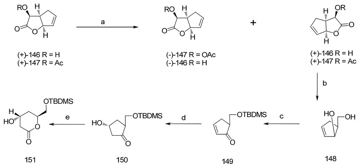
**Scheme 22.** Reagents and conditions: (a) PFL, vinyl acetate or PFL, buffer solution pH= 7; (b) (i) LiAlH<sub>4</sub>, THF, (ii) NaIO<sub>4</sub>, H<sub>2</sub>O, (iii) NaBH<sub>4</sub>; c) (i) TBDMSCl, Et<sub>3</sub>N, DMAP; (ii) PDC, CH<sub>2</sub>Cl<sub>2</sub>; (d) (i) H<sub>2</sub>O<sub>2</sub>, NaOH, MeOH, 0°C; (ii) Al(Hg), THF-H<sub>2</sub>O; (e) DCM/MCPBA.
