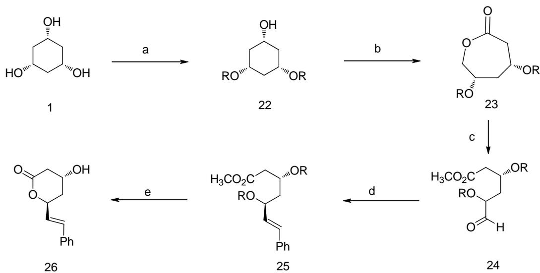
**Scheme 3.** *Reagents and conditions:* (a) (i) TBDPSCl, Imidazole, DMF; (b) (i) PCC, DCM; (ii) MCPBA, NaHCO<sub>3</sub>; (c) (i) MeOH, CF<sub>3</sub>COOH (ii) PCC, DCM; (d) (i) PhCH<sub>2</sub>=PPh<sub>3</sub>, THF; (e) (i) TBAF, THF; (ii) AcOH, THF.
