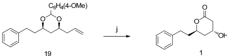
To the stirred solution of **19** (0.200 gm, 0.0006 mole) in carbontetrachloride: acetonitrile: water (1:1:2, 20 mL), NaIO<sub>4</sub> (0.256 gm, 0.0012 mole, 2 eq) and RuCl<sub>3</sub> (0.0484 gm, 0.0002 mole, 0.3 eq) were added at room temperature. The reaction mixture was stirred for 12hr. The progress of the reaction was monitored by TLC.
