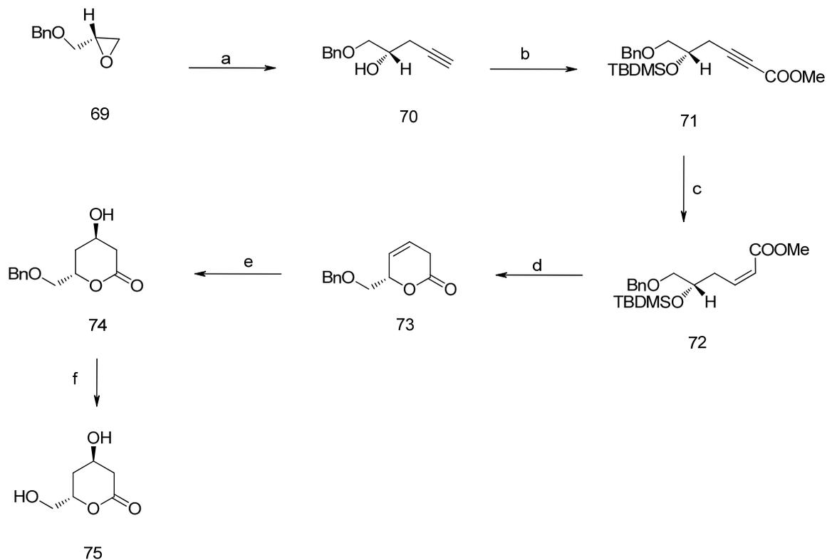
**Scheme 10.** *Reagents and conditions:* (a) (i) NaH, DMSO; (ii) Acetylene, THF; (b) (i) TBDMSCl, Imidazole, DMF; (ii) BuLi, THF,  $-78^\circ\text{C}$ ; (iii)  $\text{ClCO}_2\text{Me}$ ,  $-50^\circ\text{C}$ ; (c)  $\text{H}_2/\text{Pd}$ , quinoline, RT-1hr; (d) HCl, MeOH, RT; (e) (i)  $\text{H}_2\text{O}_2$ , NaOH, MeOH; (ii)  $(\text{PhSe})_2$ ,  $\text{NaBH}_4$ , AcOH, Iso-PrOH; (f)  $\text{H}_2/\text{Pd}(\text{OH})_2$ ,  $\text{EtOAc}_2$ , RT-1hr
