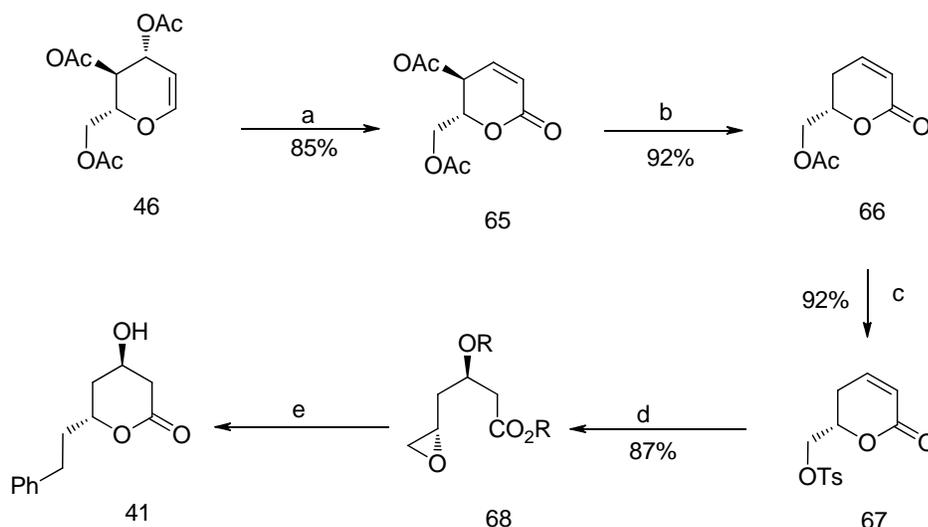
**Scheme 9.** Reagents and conditions: (a) (i) PCC, DCM, Celite; (b) (i) Zn, AcOH; (ii) TEA, RT stirring; (c) (i) 2N. HCl, (ii) TsCl, TEA; (d) (i) NaOMe/ MeOH; (e) Bn-MgCl, CuBr-Me<sub>2</sub>S, THF; (iii) 10% Pd-C, Dioxane + Water.
