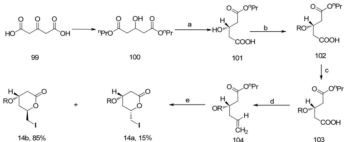
**Scheme 15.** Reagents and conditions: (a) PLE, H<sub>2</sub>O, Buffer (b) TBDMSCl, imidazole (c) (i) BH<sub>3</sub>, THF -20 to 0°C, (ii) PCC, CH<sub>2</sub>Cl<sub>2</sub> (d) (i). CH<sub>3</sub>PPh<sub>3</sub>Br, toluene KN(SiMe<sub>3</sub>)<sub>2</sub>, -15 to 0°C (ii) NaOH, EtOH, H<sub>2</sub>O (e) Et<sub>2</sub>O, NaHCO<sub>3</sub>, I<sub>2</sub> (5 eq.)
