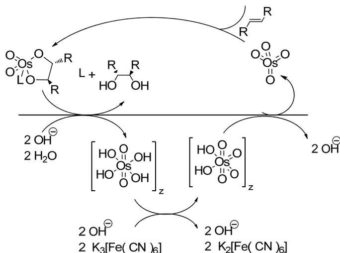
**Figure 5:** Osmium mediated 1, 2 di-hydroxylation of olefins with  $K_3Fe(CN)_6$
