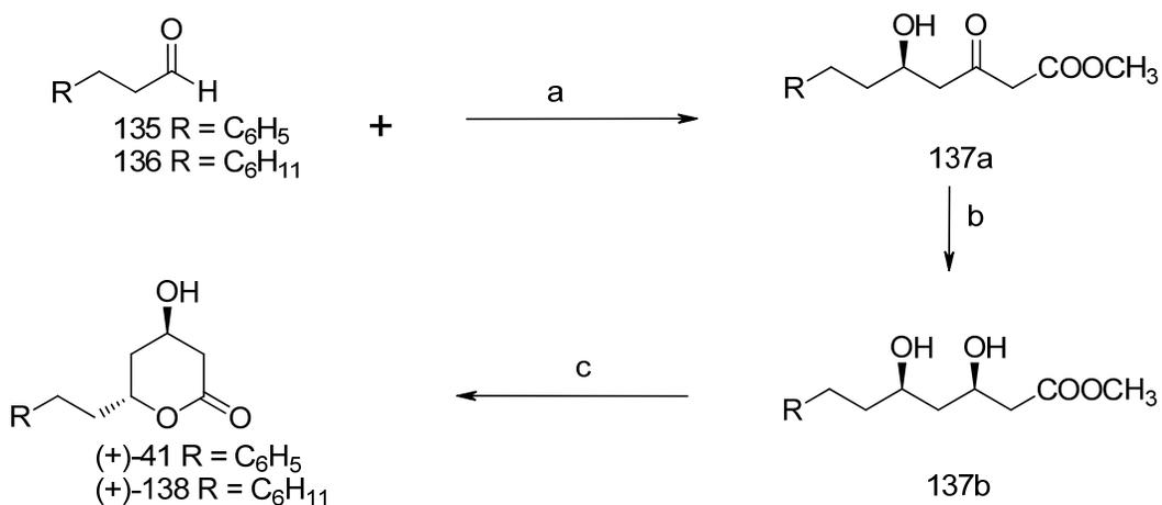
**Scheme 20.** Reagents and conditions: (a) Methyl aceto-acetate, NaH, BuLi, HMPA, THF; b) (i) Bu<sub>3</sub>B, MeOH; (ii) NaBH<sub>4</sub>; (c) PPL, ether.
