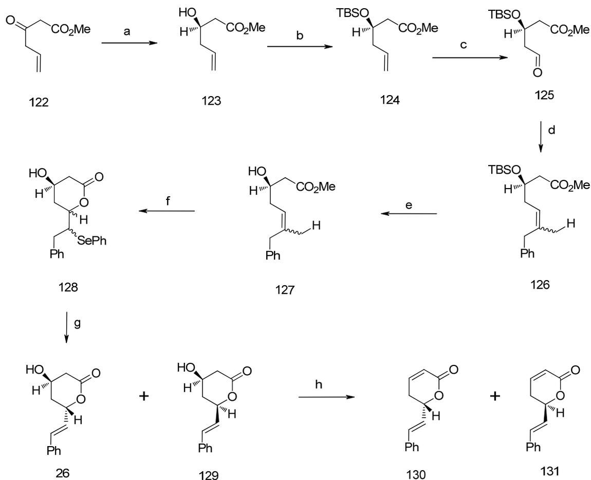
**Scheme 18.** Reagents and conditions: (a) B.Y.reduction; (b) NEt<sub>3</sub>, TBDMSCl, DCM; (c) O<sub>3</sub>, MeOH, AcOH; (d) PH<sub>3</sub>P=BnBr, THF; (e) TBAF, THF, (f) PhSeH, THF, Lactn (g) TBHP, Heat; (h) TsCl, TEA, DCM, Heat, -H<sub>2</sub>O
