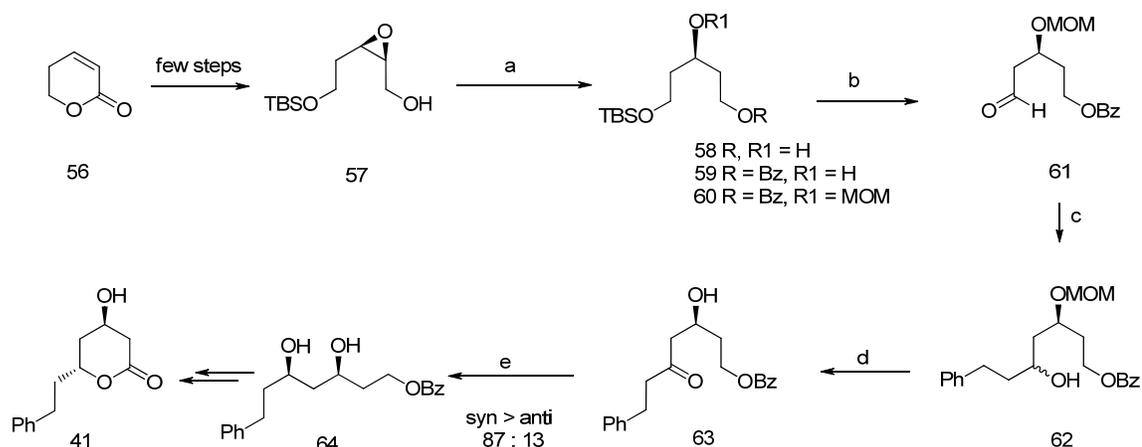
**Scheme 8.** *Reagents and conditions:* (a) Red-Al, THF, -20°C; (b) (i) TBAF<sub>4</sub>, THF; (ii) PCC, DCM; (c) BnCH<sub>2</sub>-MgBr, THF, -20°C; (d) (i) PCC, DCM; (ii) Me<sub>2</sub>BBr, THF; (e) (i) Ti-(isopropoxide)<sub>4</sub>, THF; (ii) NaBH<sub>4</sub>, THF, 80°C.
