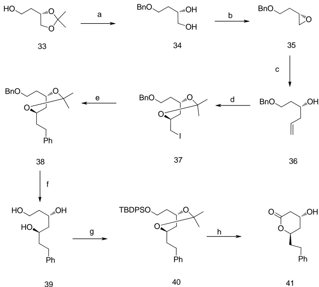
**Scheme 5.** Reagents and conditions: (a) (i) NaH, DMF, BnBr; (ii) AcOH, H<sub>2</sub>O; (b) (i) MsCl, Pyridine; (ii) Triton- B; (c) Vinyl-Mg-Br, THF, -20°C; (d) BuLi, CO<sub>2</sub>, I<sub>2</sub>; (e) Acetone, PTSA; (e) (i) BnSO<sub>2</sub>Ph-CH<sub>3</sub>/ DMF, KH, RT, 3hr; (ii) Na(Hg), MeOH; (f) TMS-I; (g) (i) TBDPSCl, Imidazole; (ii) Acetone, PTSA; (h) (i) TBAF, THF; (ii) Collins reagent; (iii) PDC, DMF (iv). HCl, DCM;
