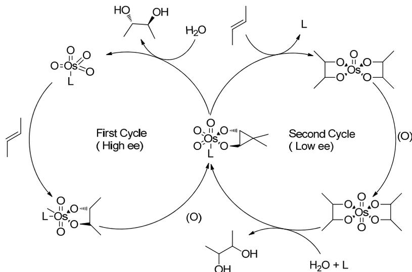
**Figure 4:** Osmium mediated 1,2-dihydroxylation of olefins with NMO as co oxidants
