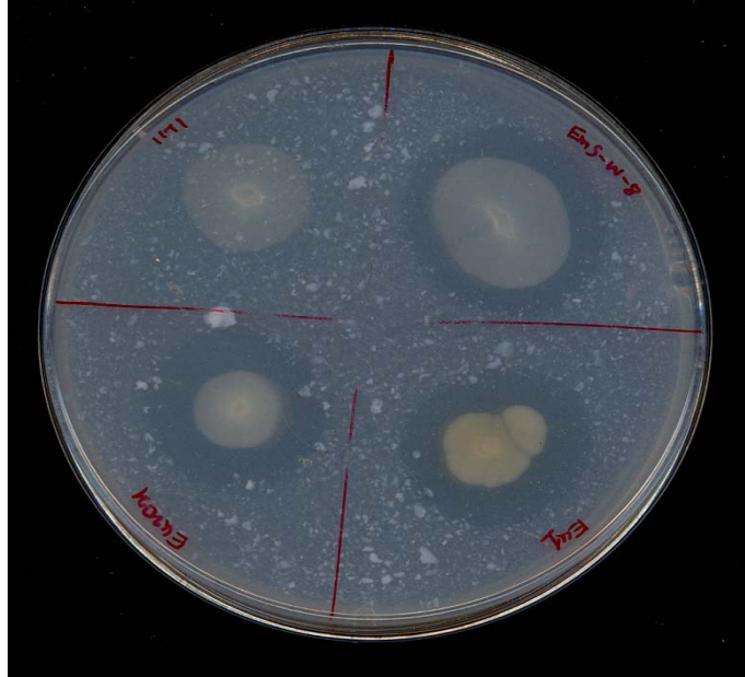
Fig. 2.2 Mutants (EMS-UV-8, EU1, and EU2D21) and parent (NCIM 1171) shows Zone of hydrolysis on plate containing 0.5% Walseth cellulose.
