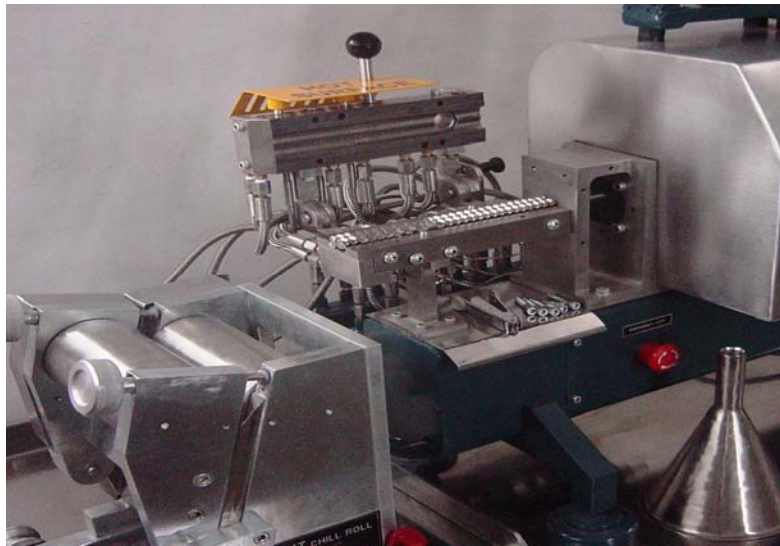
Figure 2.2 : Lab Model 16 mm Twin Screw Extruder followed by cooling, grinding and sieving(90micron sieve) for obtaining the final powder. Characterisation of these powders carried out by Differential scanning calorimetry (DSC).
