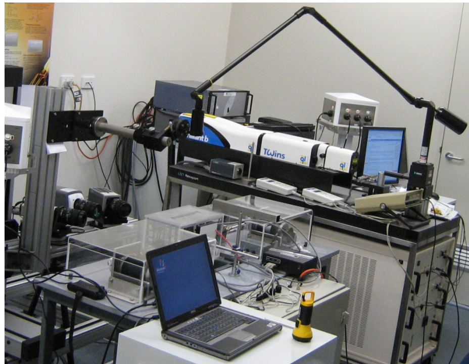
Figure 4.2 (A) Schematic of combined stereo PIV and shadowgraphy setup (B) Photograph of the setup
