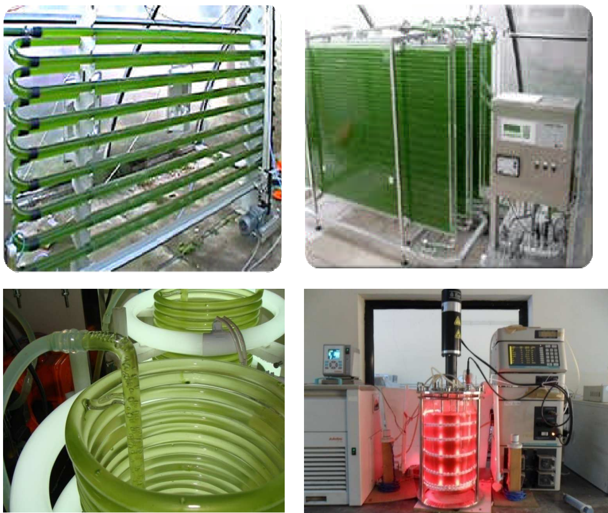
Figure 2.4: Closed photobioreactors 3A: Tubular photobioreactor, 3B: Flat plate photobioreactor, (Source courtesy for A and B photobioreactors, www. Chempuretech.com ) 3C: Helical photobioreactor, 3D: LED photobioreactor.
