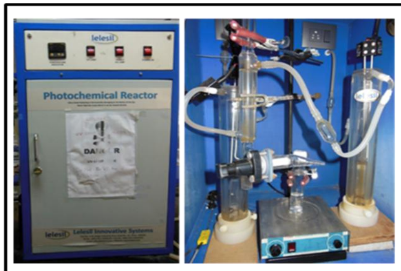
Figure 2.3. Reactor set up for photocatalytic water splitting which consists of a quartz cell having 70 ml capacity and it is gas closed by means of rubber septum. The light sources are inside the quartz jackets where cold water circulates continuously.
