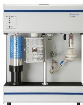
Fig. 2.3 Micromeritics Autochem 2920 used for TPD and TPR studies.
