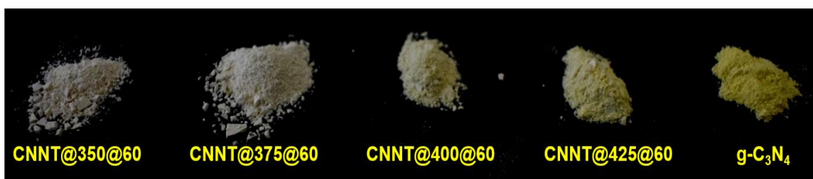
Fig. 3.4 Photograph of the catalyst with different sintered temperatures.
