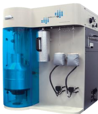
Fig. 2.2 Quantachrome Autosorb iQ instrument used for N_2 physisorption.
