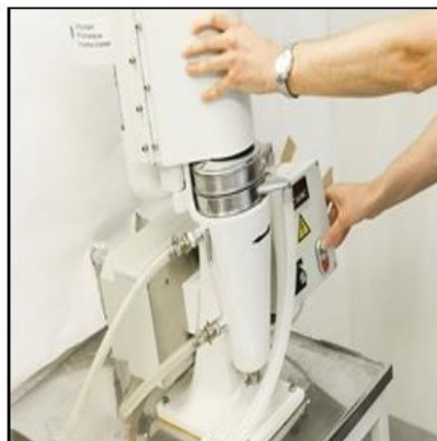
Figure 3.9: Centrifugation for biomass separation after production in fermentor
