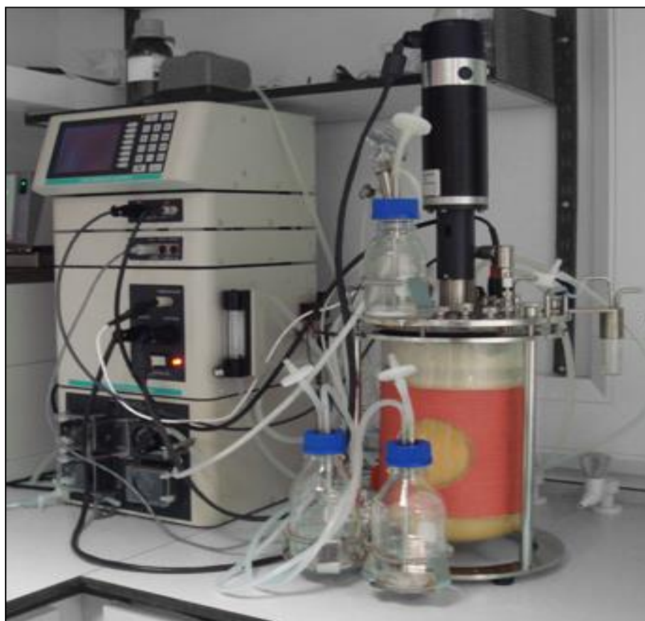
Figure 3.6: Fourteen liters fermentor in working condition
