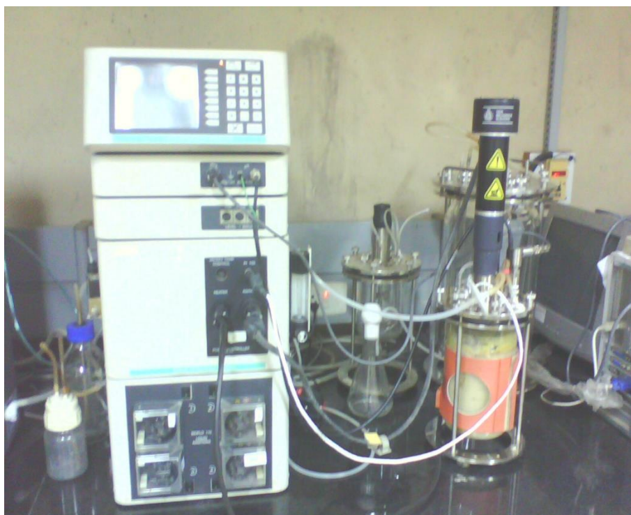
Figure 3.3: Three liters fermentor in working condition
