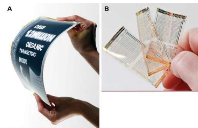
Figure 31. OFETs applications: A) Flexible electrophoretic ink display driven by an active-matrix of 1.2 million OFETs and B) Plastic foils comprising 8-bit microprocessors with 3381 OFETs each. 68
