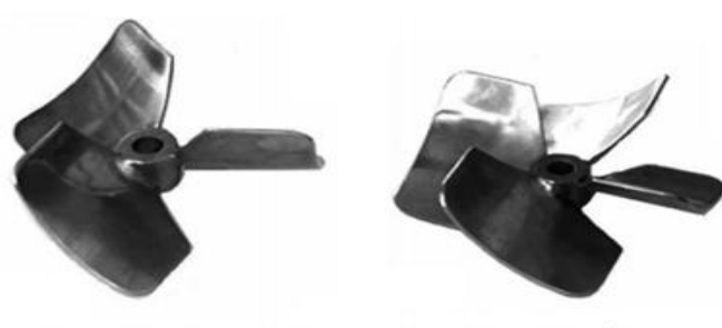
Figure 2.5: Hydrofoils with different blade angles and blade width. Reproduced with the permission from the publisher (Kumaresan and Joshi, 2006).
