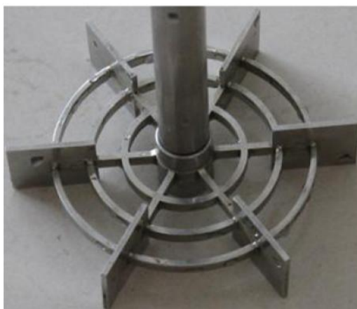
Figure 2.14: Six blade grid disc impeller (referred to as RT-G) ( Reproduced with permission from the Publisher (Yang et al., 2015)).
