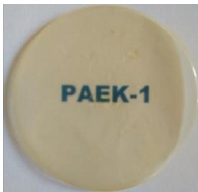
**Figure 4b.1.** Film of poly(ether ether ketone) PEEK-1.
