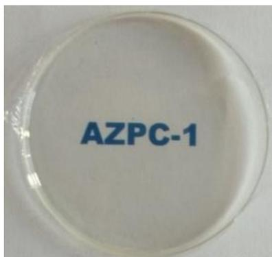
**Figure 3.5.** Film of polycarbonate AZPC-1.
