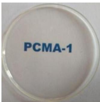
**Figure 5b.5.** Film of polycarbonate PCMA-1.
