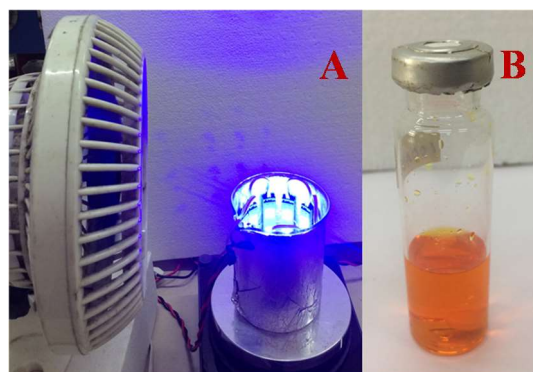
Figure 3.5. (A) Reaction setup for ADH of N -heterocycles. (B) Reaction after 12 h.
