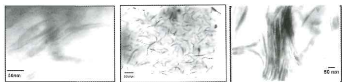
TEM micrographs of various regions of intercalated PETOB-clay nanocomposites
