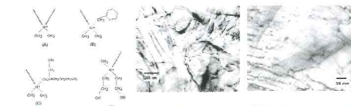
Organic modifiers used in the study and TEM micrographs of intercalated PMMA nanocomposites.
