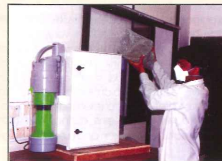
Use of mycoharvester to harvest spores of insect-pathogenic fungi
