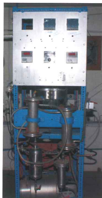
Laboratory assembly for ATR catalyst testing
