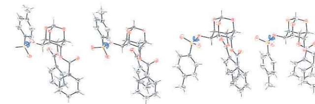
Four conformational polymorphs of (I), forms A-C occur concomitantly, all of them transform to D upon heating
