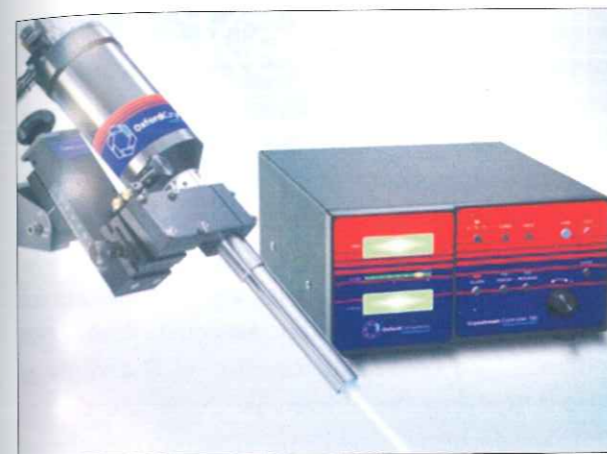
Oxford cryostream plus installed at Bruker SMART APEX single crystal X-ray diffractometer
