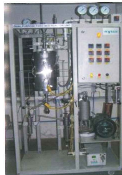
Reactor for testing of WGS monolith catalysts
