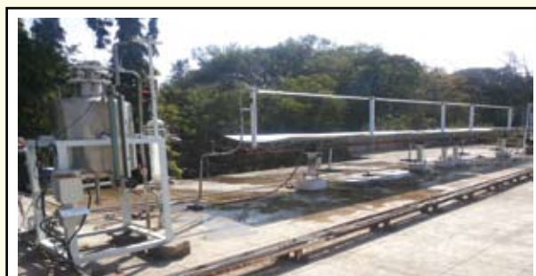
Fig. 1: Pilot scale photocatalytic reactor assembly for the treatment of industrial wastewater
