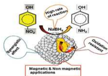
Fig. 2: The rate of p -nitrophenol reduction reaction on the as synthesized and annealed Au@Ni catalyst (both fcc and hcp). The schematic shows the diverse properties exhibited by the bimetallic nanostructures
