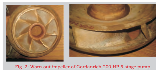
Fig. 2: Worn out impeller of Gordanrich 200 HP 5 stage pump
