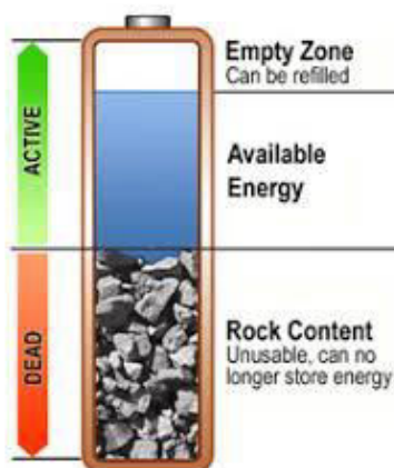
Figure 1.9: Battery energy utilization zones (Reprinted with the permission of https://batteryuniversity.com/learn/article/capacity_loss ).
