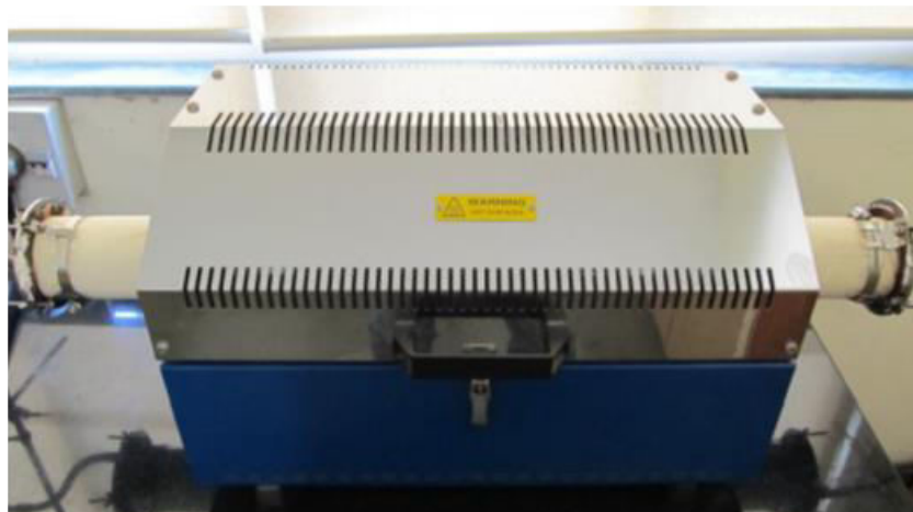
Figure 2.5: Photograph of the tubular furnace used for the synthesis of carbon materials.
