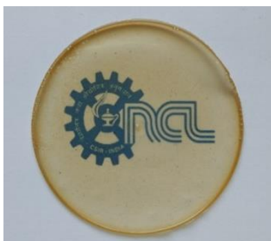
Figure 4.1. Solution casting of P19(4a-5b) to obtain a transparent film with CSIR-NCL logo in the background.
