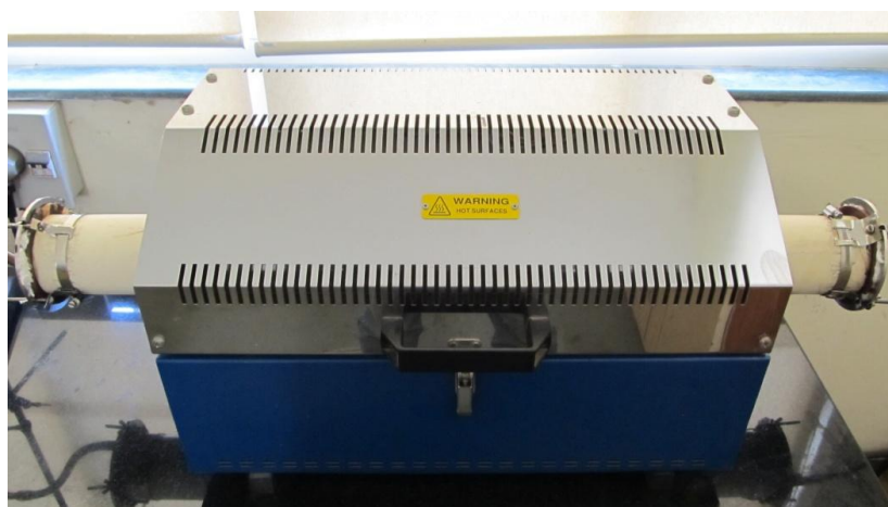
Figure 2.1 Image of a split tube furnace used for synthesis of carbon by high temperature pyrolysis
