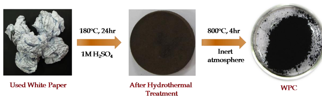
Scheme 4.1 Schematic representing the synthesis protocol for carbon from waste paper (WPC).
