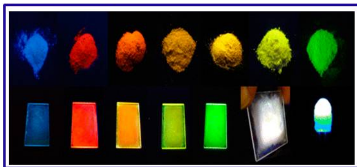
Figure 1.3: Images of luminescent materials with tunable emission colors under 254 nm UV lamp illumination (Adapted from ACS Appl. Mater. Interfaces 2014, 6, 12915).
